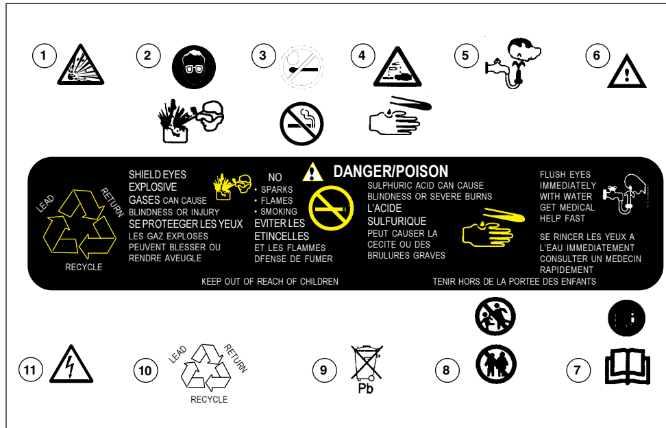
Fig. 1—Typical Battery Labelling
