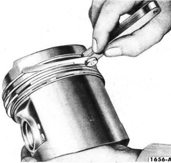
FIG. 47—Checking Ring Side Clearance
