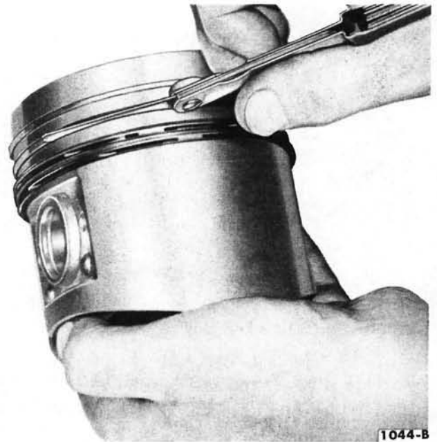
FIG. 64—Ring Side Clearance—Typical
