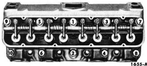
FIG. 26—Cylinder Head Bolt Tightening Sequence
