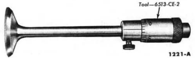
FIG. 23—Measuring Valve To Cap Clearance—Free Turning Valve
