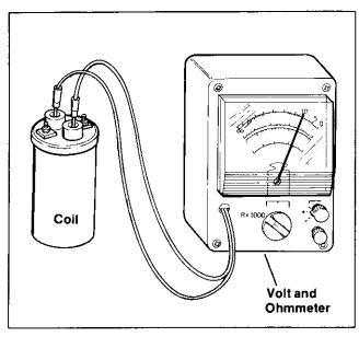
Figure 6-4. Resistance Check of Coil Secondary
