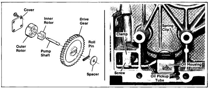
Figure 5-5. Oil Pump Assembly and Center Oil Pickup
