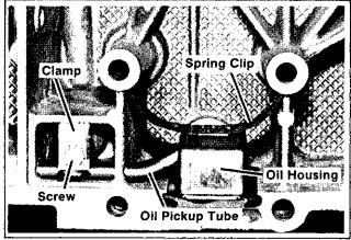
Figure 8-3. Installing Center Oil Pickup
