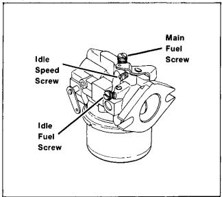
Figure 4-1. Carburetor Adjustments
