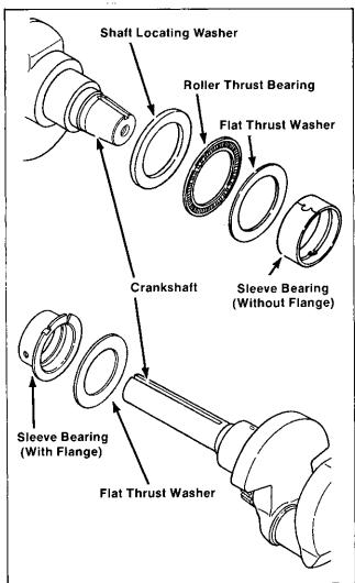
Figure 8-7. Assembly Of Roller Thrust Bearing
