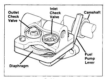
Figure 4-9. Fuel Pump Function
