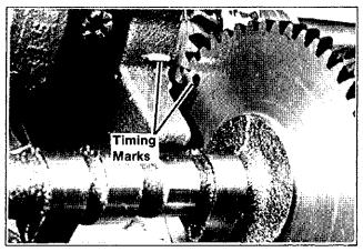
Figure 8-11. Match Timing Marks On Cam And Crank
