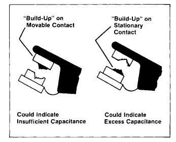
Figure 6-2. Metal Transfer On Points
