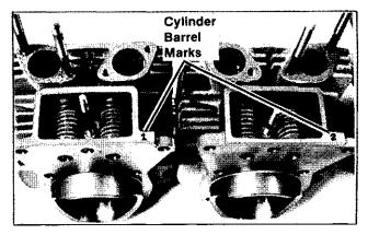
Figure 7-4. Cylinder Barrel Identification
