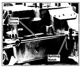
Figure 7-16. Splitting the Crankcase
