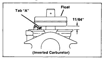
Figure 4-4. Setting Float Level
