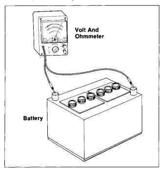
Figure 6-5. Checking Battery Charge
