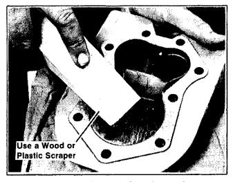
Figure 7-5. Cleaning Cylinder Heads
