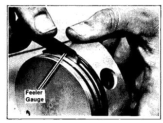
Figure 7-12. Checking Piston - Ring Side Clearance
