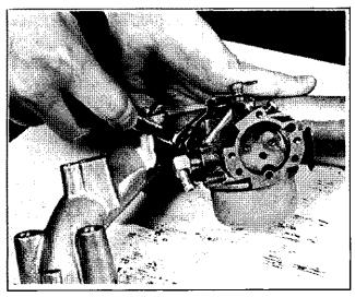
Figure 8-37. Mounting Carburetor On Intake Manifold
