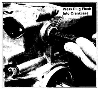
Figure 8-20. Installing Camshaft Bore Cup Plug
