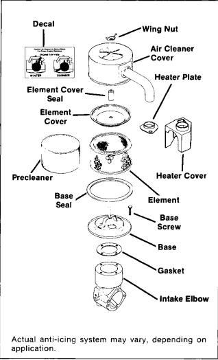
Figure 3-6. Anti-Icing System
