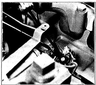
Figure 6-6. Point Gap Adjustment
