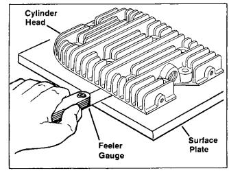
Figure 7-6. Checking Cylinder Head Flatness
