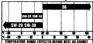
Straight 30-weight oil is recommended. Do not use multi-viscosity oils above 32°F (0°C) as considerable increases in oil consumption and combustion deposits will result.
