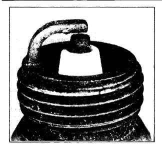
White Chalky Deposits: Overheating will be indicated by chalk white colored deposits, not burned black as might be expected. This condition is also usually accompanied by excessive gap erosion. Overadvanced timing, lean carburetion, clogged air intake and blocked cooling fins are some of the causes of overheating.
