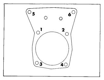
Figure 8-24. Barrel Nut Tightening Sequence
