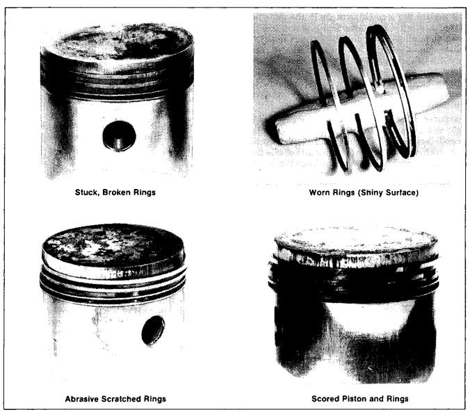
Figure 7-10. Common Sources Of Piston And Ring Damage
