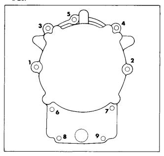
Figure 8-26. Closure Plate Screw Tightening Sequence
