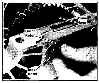
Figure 7-19. Removing Oil Pump Rotors (Early design crankcase shown).
