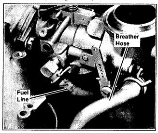
Figure 8-39. Fuel And Breather Hose Connections
