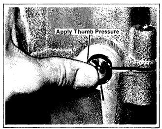
Figure 8-16. Installing #2 Crankcase Half
