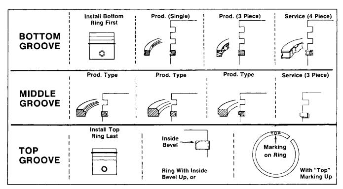
Figure 7-13. Production Type And Service Type Piston Rings
