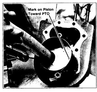
Figure 8-22. Installing Pistons In Cylinder Barrels
