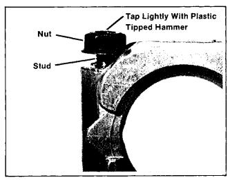
Figure 7-17. Removing Posi-Lock Connecting Rods
