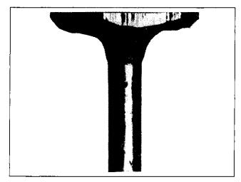
Carbon Cut: Excessive buildup of deposits in the combustion chamber may result in valve damage because deposits can become hard enough to cut the valve. Cleaning of the cylinder head at proper intervals could prevent such damage.
