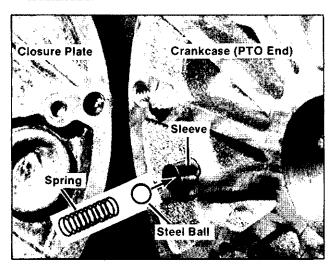
Figure 8-25. Installing Oil Pressure Relief Valve
