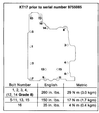
Figure 8-18. Crankcase Torque Sequence.
