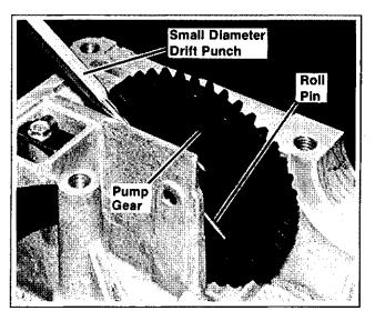
Figure 7-20. Removing the Oil Pump Gear
