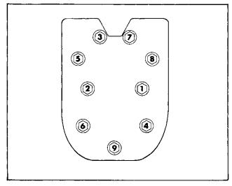
Figure 8-28. Cylinder Head Screw Tightening Sequence
