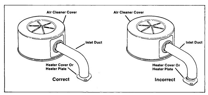
Figure 3-8. Installing Anti-Icing Air Inlet Duct
