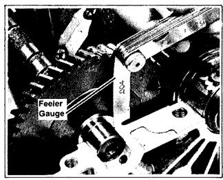
Figure 8-12. Checking Camshaft End Play
