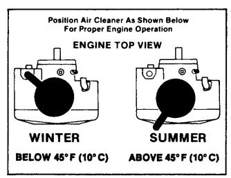
Figure 3-7. Typical Anti-Icing Air Cleaner Cover Positions
