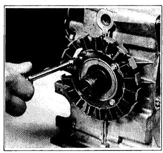
Figure 8-21. Installing Stator.
