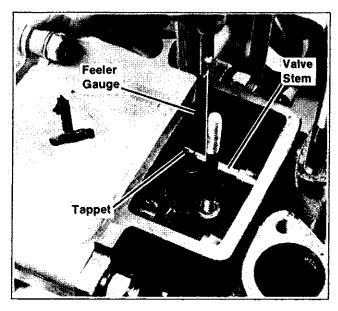
Figure 8-27. Checking Valve Clearance
