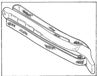
Figure 1-3. Flywheel Strap Wrench (52 455 03) Replacement Strap (52 445 04)
