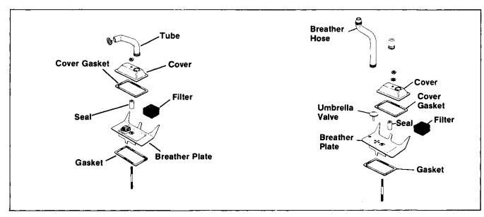
Figure 8-29. Exploded View Of Breather Components (Early Design On Left)
