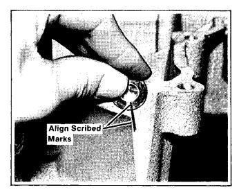
Figure 8-15. Installing Machined Camshaft Bore Plug Into #1 Half
