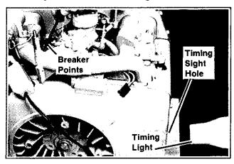
Figure 6-7. Timing Light Method
