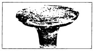
Bad Condition: The valve depicted here should be replaced. Note the warped head; margin damaged and too narrow. These conditions could be attributed to excessive hours or a combination of poor operating conditions.
