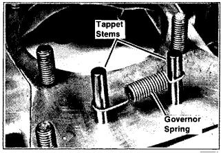
Figure 8-10. Use Governor Spring to Hold Tappets (#2 Side)
