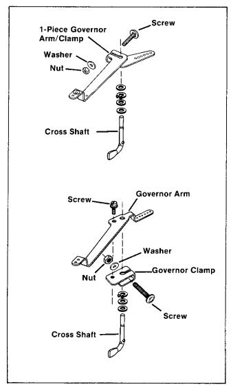
Figure 8-40. Installing Governor Arm
