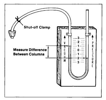
Figure 1-5. "U" Tube Manometer
