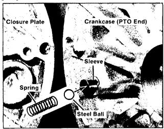
Figure 5-3. Oil Pressure Relief Valve
