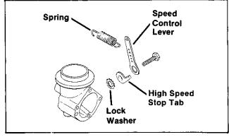
Figure 8-38. Assembling Governor Speed Control Lever
