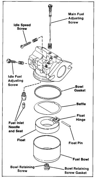
Figure 4-2. Side Draft Carburetor - Exploded View
