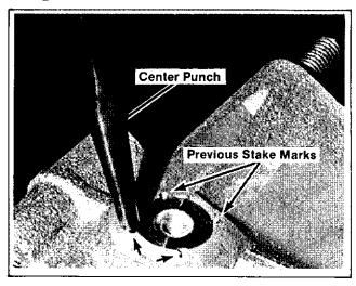
Figure 8-19. Restaking Camshaft Bore Plug.
