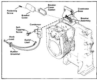
Figure 8-42. Condenser Assembly
