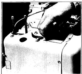
Figure 8-33. Attaching Cylinder Head Baffles
