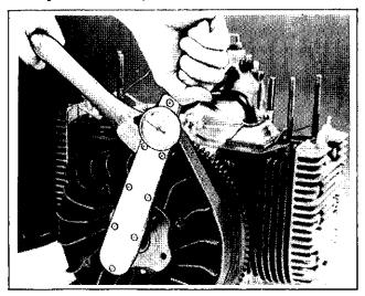
Figure 8-32. Torquing Flywheel Retaining Screw
