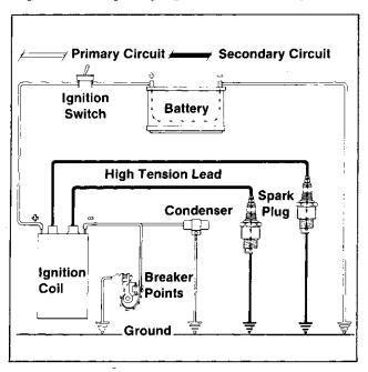
Figure 6-1. Schematic of a Typical Battery Ignition System
