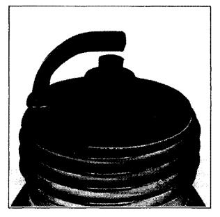
Carbon: Soft, sooty black deposits indicate incomplete combustion which could be attributed to rich carburetion, weak ignition, retarded timing or poor compression.
