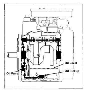
Figure 5-1. Pressurized Spray Lubrication System
