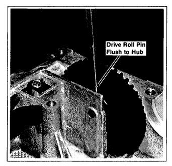
Figure 8-4. Securing Oil Pump Gear To Shaft
