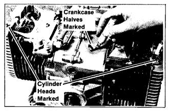
Figure 7-3. Marking The Case Halves For Identification
