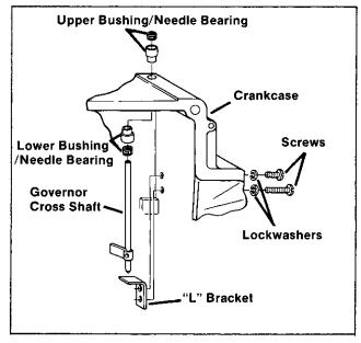
Figure 8-2. Installing Governor Cross Shaft— Generator Applications
