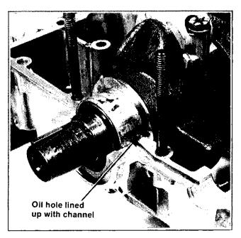
Figure 8-8. Position Of The Bearing To The Crankcase
