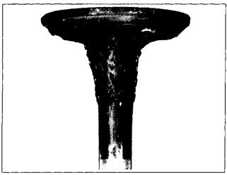
Gum: Gum deposits usually result from using stale gasoline. This condition is often noted in applications where fuel is not drained out of tank during the off season. Gum is a prevalent cause of valve sticking. The cure is to ream the valve guides and clean or replace the valves, depending on their condition.
