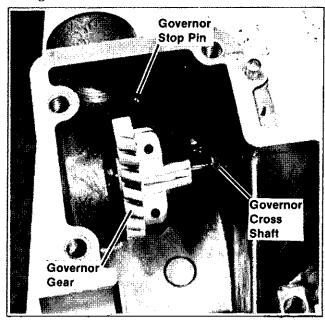
Figure 8-1. Governor Gear And Cross Shaft - Installed
