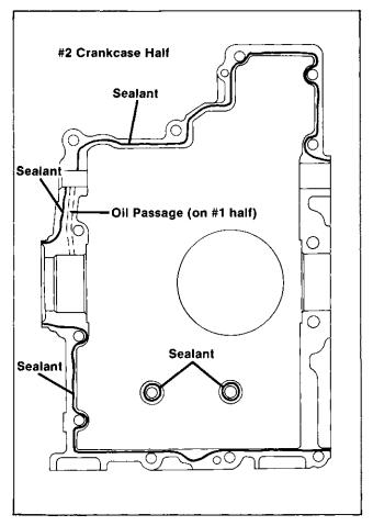
Figure 8-14. Applying Crankcase Sealant
