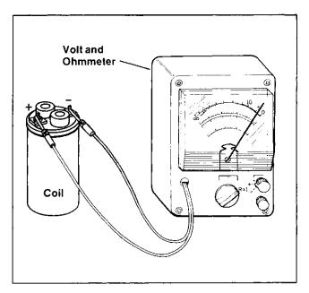
Figure 6-3. Continuity Check of Coil Primary
