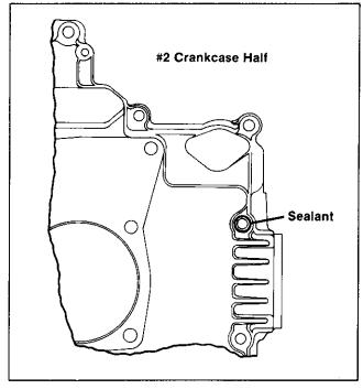
Figure 8-13. Applying Crankcase Sealant-Crankcase Exterior
