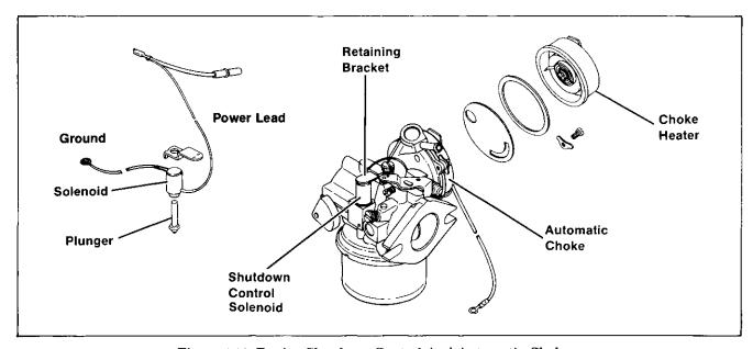
Figure 4-11. Engine Shutdown Control And Automatic Choke
