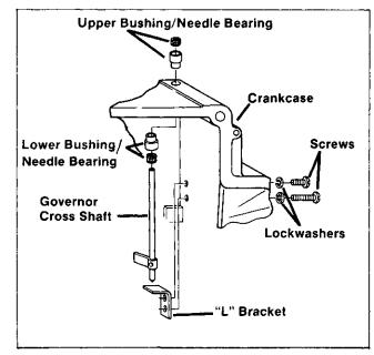
Figure 7-18. Removing Governor Cross Shaft— Generator Applications
