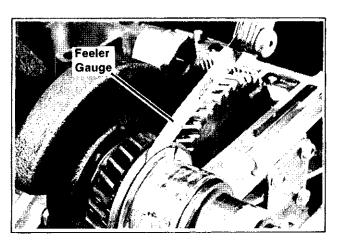
Figure 8-9. Checking Crankshaft End Play
