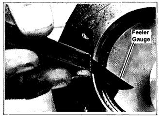
Figure 7-11. Checking Ring End Gap In Bore
