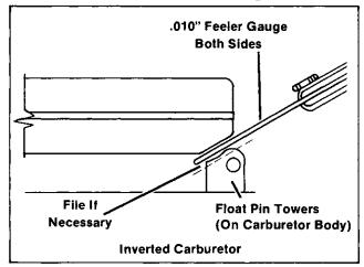
Figure 4-6. Checking Float Clearance
