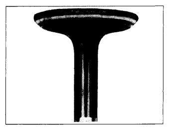
Overheating: An exhaust valve subject to overheating will have a dark discoloration in the area above the valve guide. Worn guides and faulty valve springs may cause this condition. Also check for clogged air intake, blocked fins, and lean fuel mixture when this condition is noted.
