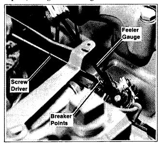
Figure 8-36. Adjusting Breaker Points
