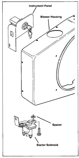
Figure 8-34. Mounting Ignition Switch And Starter Solenoid
