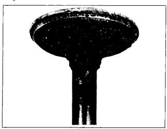
**Coking:** Coking is normal on intake valves and is not harmful. If the seat is good, the valve could be reused after cleaning.
