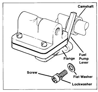
Figure 8-30. Installing Fuel Pump
