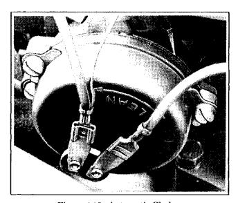
Figure 4-10. Automatic Choke.
