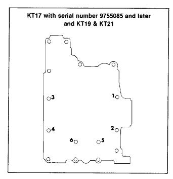
Figure 8-17. Crankcase Torque Sequence.
