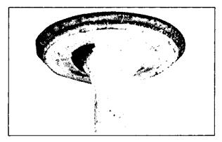
Normal: Even after long hours of operation a valve can be reconditioned and reused if the face and margin are in good shape. If a valve is worn to where the margin is less than 1/32" do not reuse it. The valve shown was in operation for almost 1000 hours under controlled test conditions.
