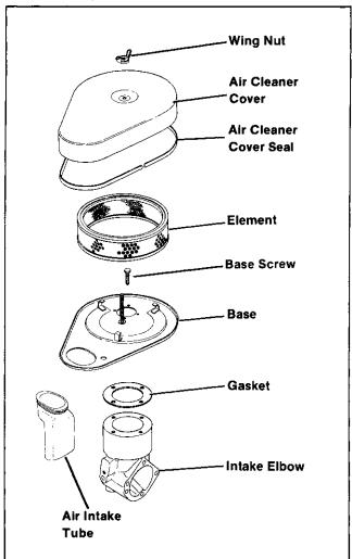
Figure 3-1. Tear Drop Air Cleaner Assembly
