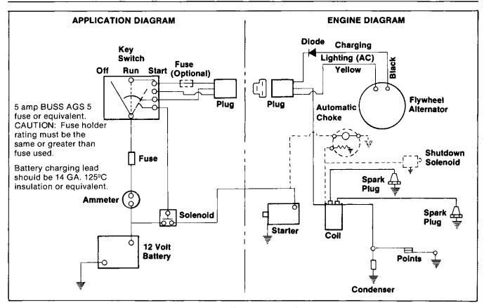
Figure 6-8. 3 Amp System Wiring Diagram
