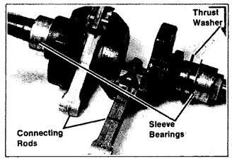
Figure 8-6. Crankshaft Components Assembled (Sleeve Bearings Shown)
