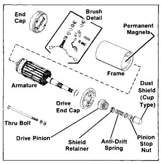
Figure 6-10. Components of Permanent Magnet Starter
