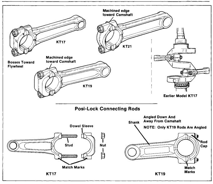
Figure 8-5. Note Differences In Connecting Rod Design
