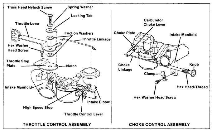
Figure 4-8. Engine Throttle And Choke Controls
