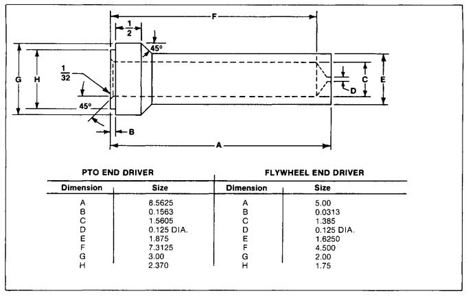
Figure 1-6. Seal Driver (P.T.O.)—Seal Driver (Flywheel)
