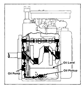
Figure 5-2. Full Pressure Lubrication System
