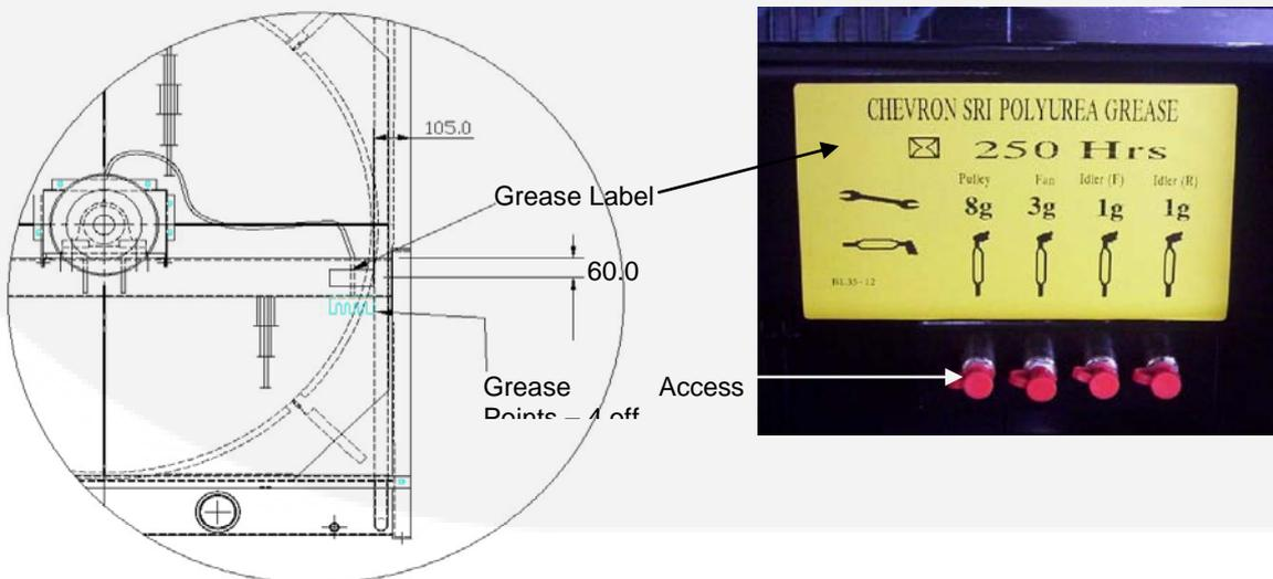
Grease quantity and greasing intervals have been designed to coincide with engine service intervals. This will prevent over greasing (it is possible to hydraulically lock a bearing by over greasing a stationary bearing).
