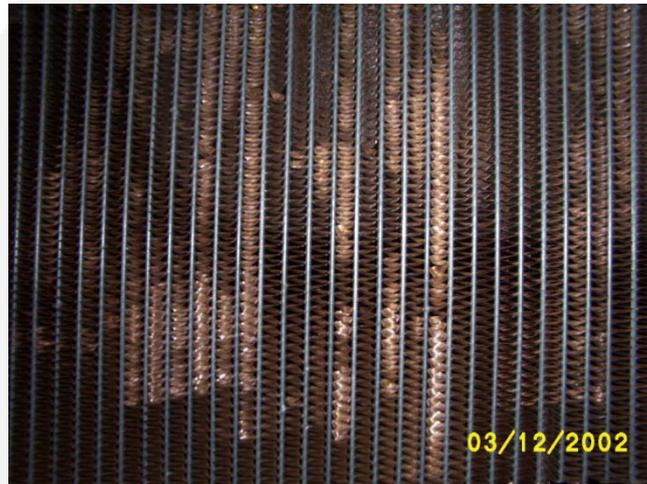
Figure 2-1 *Fins damaged by compressed air at acute angles to core face*
