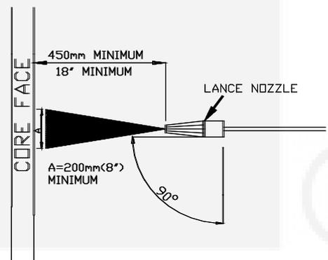
**Note:** *If your pressure washer works above 3000 PSI then the gap between the nozzle and the core face must be increased or fin damage will occur.*
