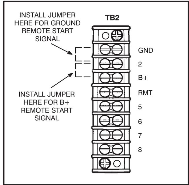
FIGURE 3-4. TB2: TWO-WIRE START CONNECTIONS
