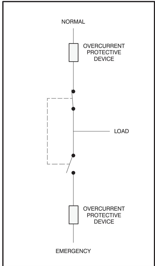
FIGURE 1-1. LOAD TRANSFER PANEL (TYPICAL FUNCTION)
