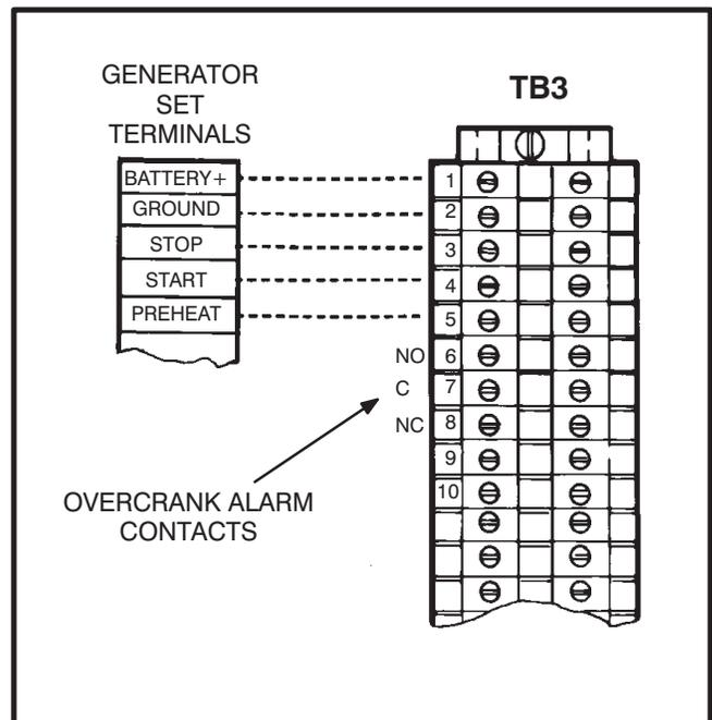
FIGURE 3-5. THREE-WIRE START CONNECTIONS
