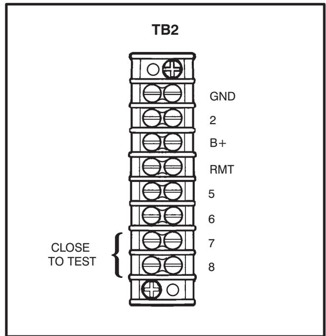
FIGURE 3-6. TB2: AREA PROTECTION / REMOTE TEST
