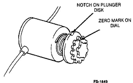
At this position there is no fuel flow when the Auto Prime is energized. To start and increase fuel flow, turn dial clockwise while manually depressing plunger.
