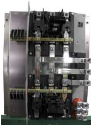
FIGURE 7a – 3-pole transfer switch (partially assembled)
