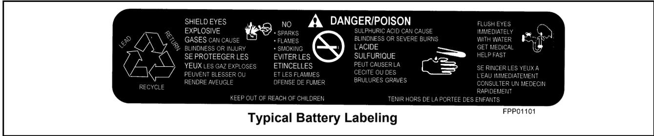
The handling and correct use of lead acid batteries is not as hazardous provided that sensible precautions are observed and that operatives have been trained in their use and are adequately supervised. It is important that all labeling on the battery is carefully read, understood and complied with. The format of the following symbols and labels is common to most brands of lead acid battery.
