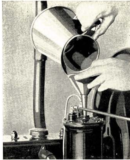
Figure 11 Filling Vacuum Tank
