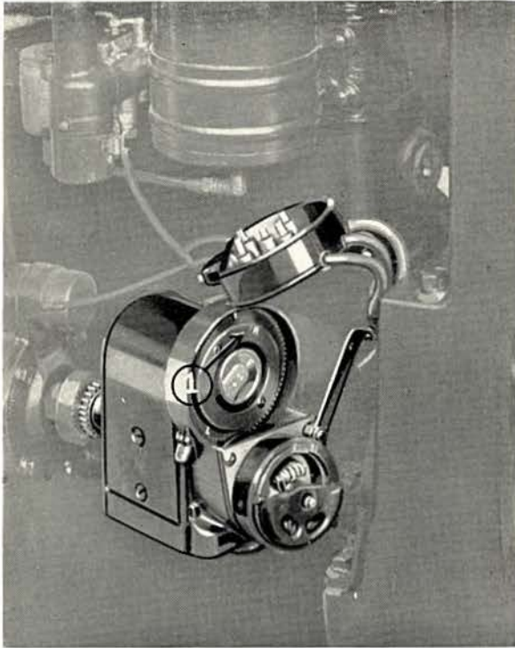
Figure 19 Timing Ignition—Magneto Setting Showing (1) Setting Notch
