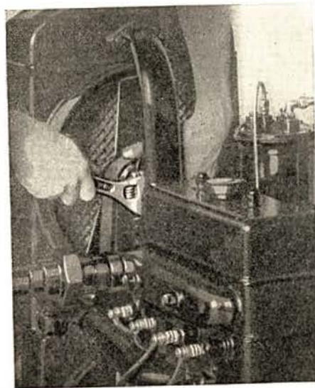
Figure 27 Adjusting Fan Belt
