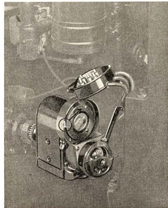
Figure 28 Timing Ignition—Magneto Setting Showing Setting Notch (1)
