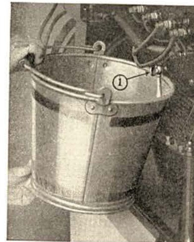
Figure 30 Draining Water Showing Water Drain Cock (1)
