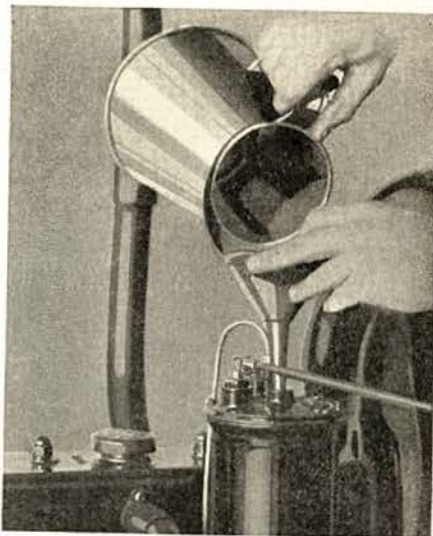
Figure 12 Filling Vacuum Tank
