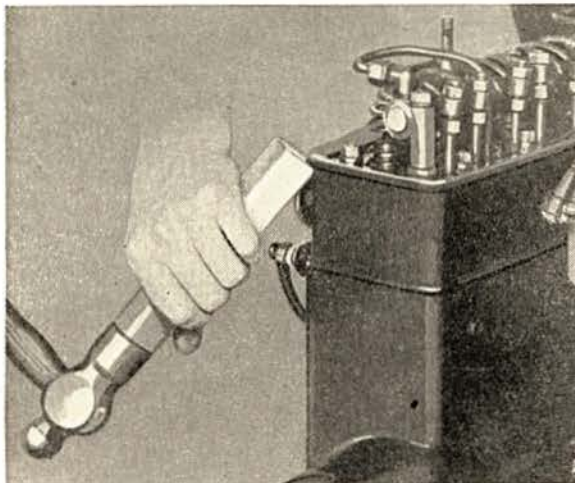
Figure 24 Loosening Cylinder Head by Tapping
