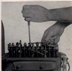
Figure 19 Adjusting Valve Clearance
