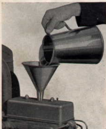
Figure 6 Filling Oil Base (Capacity 7 Quarts.)
