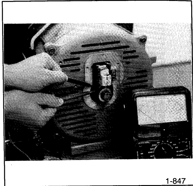
Figure 7-6. Rotor Resistance Check
