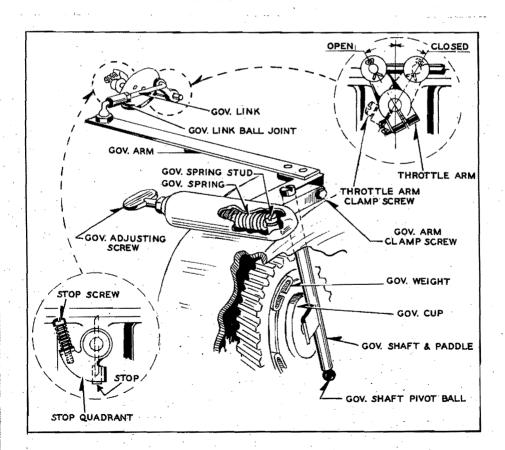
The governor arm is linked to the carburetor throttle arm. This, whenever the load changes and the speed tends to gain or drop, the governor mechanism immediately moves to offset the change in load and either opens or closes the throttle valve to compensate for the change.
