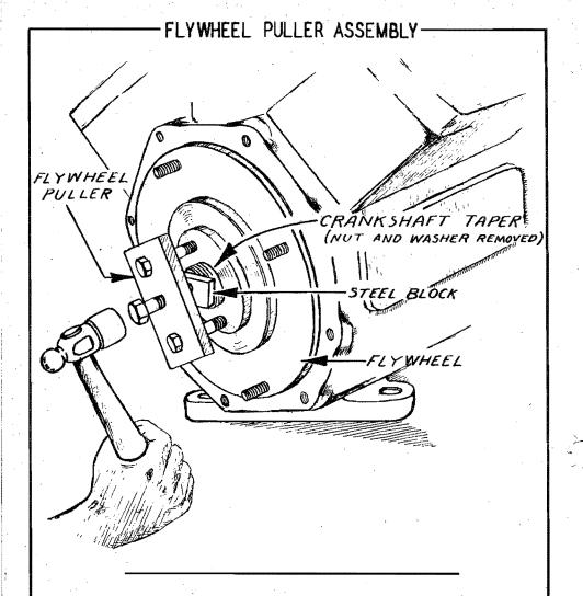
THE REAR ENGINE VIEW SKETCH ABOVE ILLUSTRATES THE OPERATION OF THE FLYWHEEL PULLER IN REMOVING THE FLYWHEEL FROM THE CRANKSHAFT TAPER.
