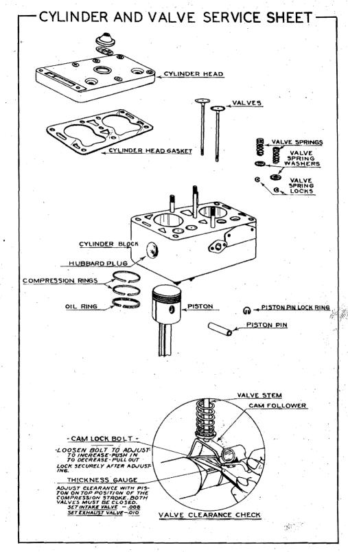
Each year, if the plant is used under normal conditions the accumulated hours of operation will total 2500 or more. After every 2500 to 3000 hours, the engine should be given a thorough checking over, the valves should be ground, the carbon removed, and the pistons, piston rings, valves, bearings, etc. should be carefully checked.
