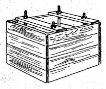
A form should be built into which the concrete can be poured and allowed to harden. The form should be large enough so base will be of the minimum size.
