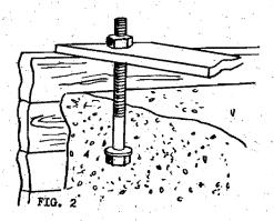
Suspend mounting bolts from cross cleats nailed to the top of the concrete form before bouring concrete. Place large washer under head of bolt and adjust for proper height - 3-1/2m
