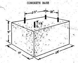
Above base dimensions are a minimum and may be larger. Keep same bolt spacing. The base must be at least 24" from any wall.
