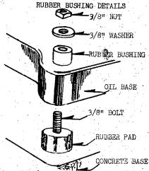
Use the rubber mounting bushings supplied with the plant.
