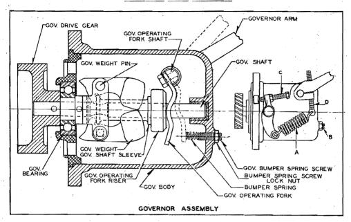
A Pierce industrial type governor is bolted to the top of the gearcase cover where it is driven by the camshaft timing gear. There is no routine servicing required for this governor. In fact, it should never need attention unless the engine has been overhauled.
