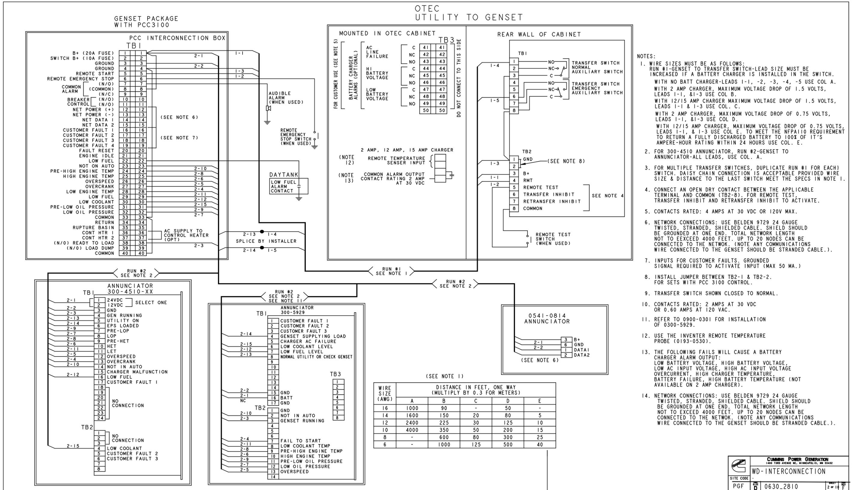
**FIGURE 10. TYPICAL INTERCONNECTION WIRING DIAGRAM (WITH PCC3100)**
