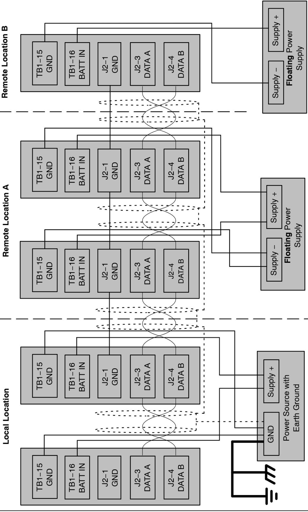
FIGURE 3. MULTIPLE REMOTE CONTROLLERS WIRING DIAGRAM
