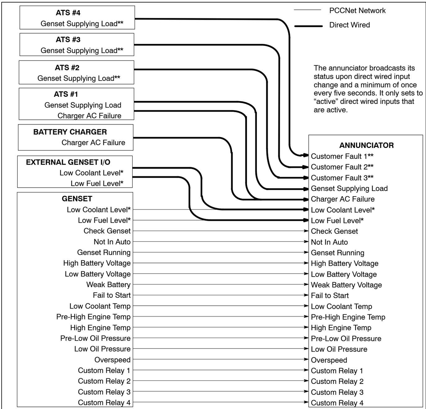
\* Low Coolant Level and Low Fuel Level statuses can be either direct wired from External Genset I/O or be part of the PCCNet network status coming from the genset. If direct wired, then the annunciator sets the appropriate bit for the genset to reference.
