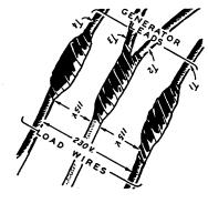
wires, one to each of the T1 and T4 generator leads. Two 115 volt circuits are thus available, one between T1 and T2, T3 and the other between T4 and T2, T3. One half the capacity of the generator is available on each circuit. Do not attempt to take the entire generator capacity from one 115 volt circuit, as the generator will be unbalanced and overloaded. Divide the load as equally as possible between the two circuits.
