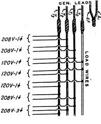
For 208 volt, I phase current, the TO generator lead is not used. Connect separate load wires to any two of the TI, T2 or T3 generator leads. Three separate single phase circuits are available T1 - T2, T1 - T3 and T2 - T3. As when connected for 120 volts, the load should be divided between the three single phase circuits.
