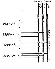
For single phase current, connect a separate load wire to each of any two generator leads. Three separate single phase circuits are thus available T1-T2, T2-T3, and and T - 3. Not more than one third of the generator capacity is available on each single phase circuit.
