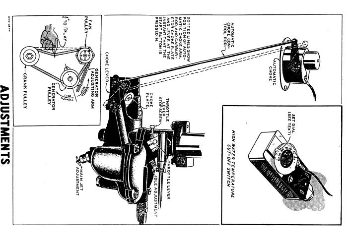
AUTOMATIC CHOKE. - The choke control should not need seasonal adjustments but may be adjusted in the following manner.
