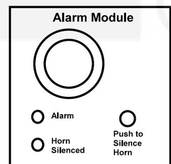
Figure 3-2 Alarm Module Front Panel
