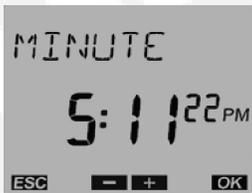
11. Press the - or + push buttons until the correct minute is displayed. Press the OK push button. The screen then shows the automatic summer/winter (SU--WI USA) time changeover flashing.
