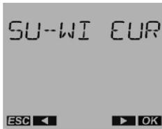
If you do not wish to set the clock for automatic Summer/Winter changeover, press the - or + push buttons. "No SU/WI" is displayed on the screen. Press the OK button to return to the SU-WI menu. SU value will flash.
