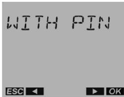
6. Press the OK push button to display the CURRENT PIN (here 0000). Continue with the OK push button.
