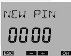
8. Press the - or + buttons to enter the first digit of the PIN code and confirm with the OK push button.
