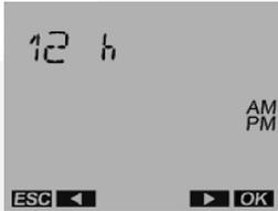
9. Press the OK push button when the desired Time format is displayed. The screen then shows the HOUR value flashing.
