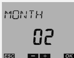
10. Press the - or + push buttons to set the correct Month. Press the OK push button to display the DAY menu. Day value will flash.
