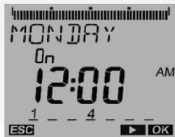
4. Press the OK push button to modify the Monday switch-on time. The MODIFY HOUR menu is displayed. The hour value will flash.
