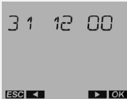
4. Press - or + push buttons to select the desired date format, then press the OK push button. The YEAR is displayed.
