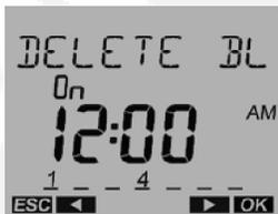
6. Press the + push button to remove MONDAY specifically from the block and delete it. The number in the lower part of the screen will flash.
