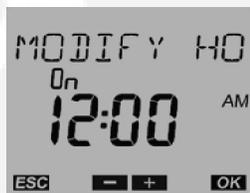
5. Press - and + push buttons to modify the hour. Press the OK push button to display the MODIFY MINUTE menu. The minute value will flash.
