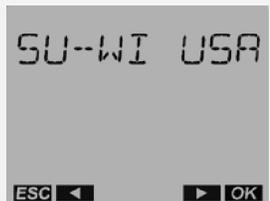
14. Press - or + push buttons to select one of the world areas that has been programmed for automatic time correction or else set up your own changeover times. Then press the OK push button to activate and return to SU-WI menu.
