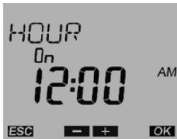
6. With the arrow push buttons - and +, set the MINUTES for the switch-on (00 minutes) and confirm with the OK push button. The minute value will flash.
