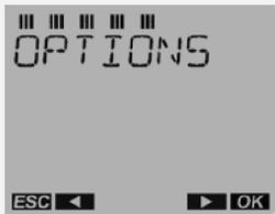
3. Press the OK push button, then press the + push button until the PIN menu appears.
