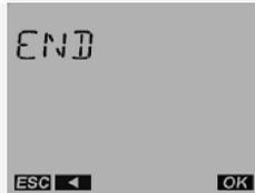
10. Press the OK push button or the MENU (ESC) push button to exit the menu.
