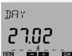
7. Press the - or + push buttons until the correct DAY is displayed and then press the OK push button. The screen then shows the FORM TIME menu.
