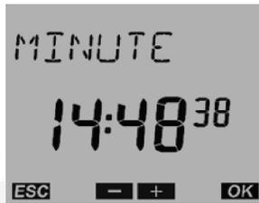
6. Press the – or + push buttons to set the correct Minute. Press the OK button to display the TIME menu.
