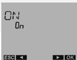
5. With the arrow push buttons - and +, set the HOUR for the switch-on (12:00 AM) and confirm with the OK push button. The hour value will flash.
