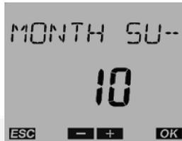
21. Press the OK push button to display the menu for setting the week when the winter changeover will take place. Press the - or + push buttons until the desired week ( 1 to 5 [1 = first week, 4 = fourth week, 5 = last week]) is displayed.
