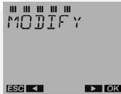
3. Press the OK push button. Now all programmed switching times are displayed classified on the time bar according to the time sequence starting with the first weekday (e.g. MONDAY). The number in the lower left will flash.
