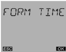
8. Press the OK push button. Press - or + to select the desired Time Format.
