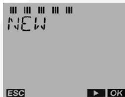
13. Press the OK push button. A brief fade-in now occurs which is only for the programming of the free memory locations. The number of available programmable time periods (maximum of 55) is temporarily displayed. This fade-in can be prematurely ended by pressing the OK push button.
