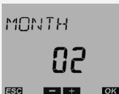
6. Press the - or + push buttons until the correct month is displayed and then press the OK push button. The screen then shows the DAY value flashing.
