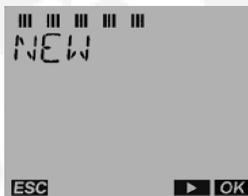
3. Press the OK push button. A brief fade-in now occurs which is only for the programming of the free memory locations. The number of available programmable time periods (maximum of 56) is temporarily displayed.
