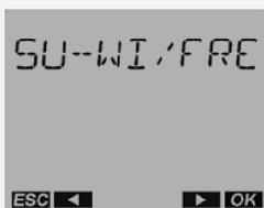
16. Press the OK push button to display the menu for setting the month when the summer changeover will take place. Press the - or + push buttons until the desired MONTH is displayed. The month value will flash.
