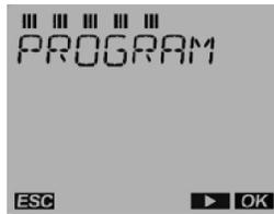
2. Press the OK push button. Press + push button twice to display the MODIFY menu.
