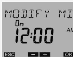
6. Press - and + push buttons to modify the minutes. Press the OK push button to display the MODIFY BLOCK menu. The numbers at the bottom of the screen will flash.
