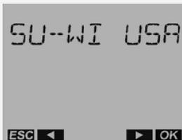
12. Press the - or + push buttons until the correct summer/winter time changeover is displayed. Press the OK push button. The time switch is now in auto mode and screen displays the correct date and time.
