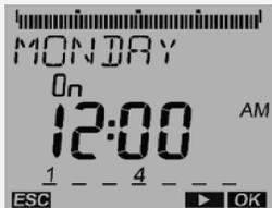
5. Press the OK push button to display the DELETE BLOCK menu. The entire switching time block (switch on at 9:00 AM from Monday to Sunday) can be deleted. The numbers at the bottom will flash.
