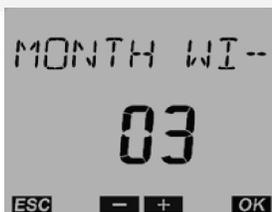
17. Press the OK push button to display the menu for setting the week when the summer changeover will take place. Press the - or + push buttons until the desired week (1 to 5 [1 = first week, 4 = fourth week, 5 = last week]) is displayed. The week value will flash.
