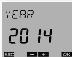
9. Press the - or + push buttons to set the correct year. Press the OK push button to display the MONTH menu. Month value will flash.
