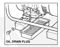
Use fresh and high quality lubricating oil to the specified level as directed on page 8. If contaminated or deteriorated oil is used or the quantity of the engine oil is not sufficient, the engine damage will result and its life will be greatly shortened.
