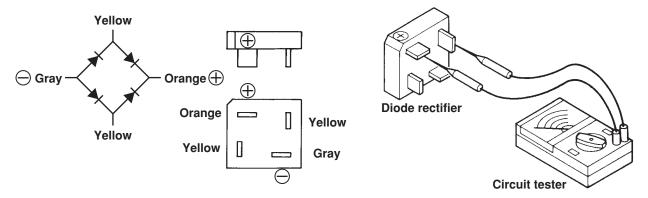
The circuit inside the diode rectifiers is as shown in the chart above.
