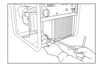
(2) Assemble the Front Cover (Lower) below the Front Cover (Upper)
