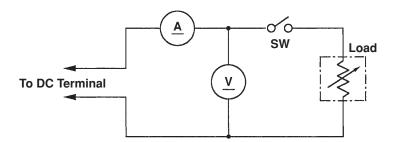
Measurement of DC output is executed with the switch turned ON while the current is regulated at 8.3A by adjusting the load to the generator. If the voltage is within the range from 6V to 14V, the voltage output is normal.
