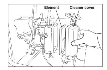
(2) Loosen the two M6 nuts and one M6 bolt, and remove the air cleaner body.
