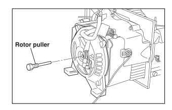
NOTE 1: Usually, you do not need to separate the rotor from the stator. However, should it be necessary, use a hand-pressing machine to press out the rotor shaft from the bearing.
