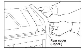
(2) Install the Muffler Cover (Rear) onto the Rear Cover (Upper) and the frame.
