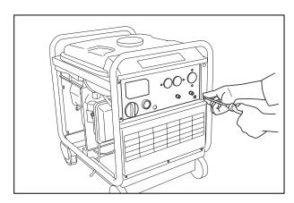
(3) Loosen the five bolts and remove the cover bracket from the inverter unit.
