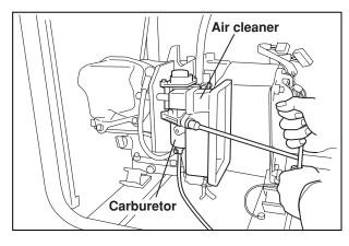
(3) Using caution not to break the gasket, carefully remove the carburetor from the insulator.
