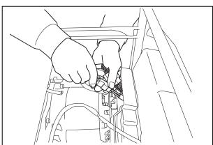
(3) For electric start models, remove the regulator mount bolt, and disconnect the wire harness from the starter motor.
