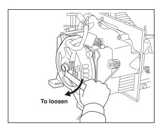
(2) Using a special tool, Rotor Puller, remove the rear cover together with rotor and stator.
