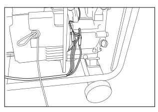
(2) Disengage the couplers of wire harness from the control panel, inverter unit and the alternator.
