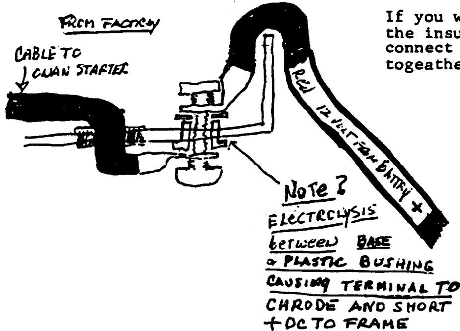
If you wish you can remove the insulated bushing and connect the positive cables together as in the inst.
