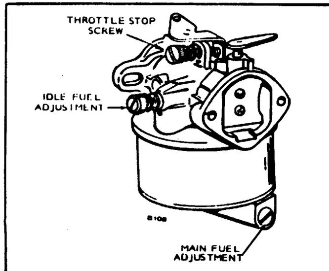
FIGURE 13. CARBURETOR ADJUSTMENTS
