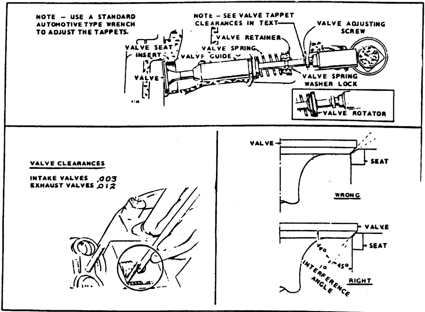
FIGURE 18. VALVE DETAILS AND CLEARANCES
