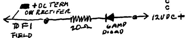
USE THIS MOMENTARILY TO FLASH FRAME FIELD TO START GENERATING CURRENT FROM GENERATOR ARMATURE SLID RINGS SOMETIMES FIELD ARMATURE LOSES MAGNETISM DUE TO LONG STORAGE + NEEDS TO BE SHOCKED TO PRODUCE A DC FIELD AROUND ARMATURE
