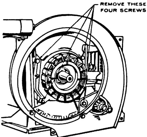
FIGURE 42. REMOVING BACKING PLATE
