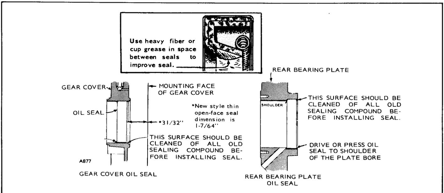
FIGURE 20. GEAR COVER AND REAR BEARING PLATE OIL SEALS
