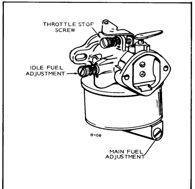
FIGURE 33. CARBURETOR ADJUSTMENTS
