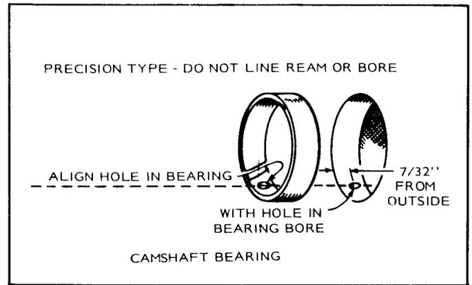
FIGURE 15. CAMSHAFT BEARING
