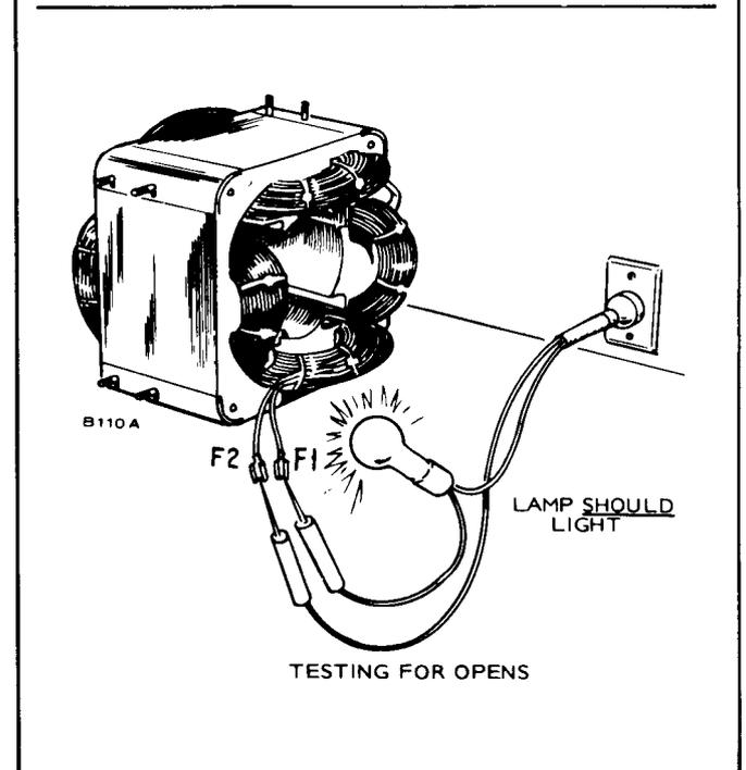
FIGURE 53. TESTING FIELD WINDINGS
