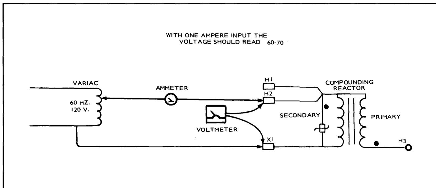
FIGURE 56. TESTING COMPOUNDING REACTOR
