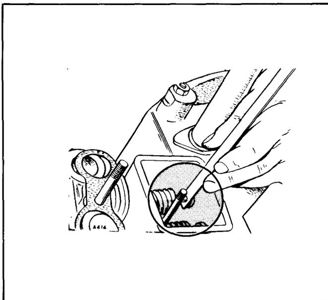
FIGURE 2. ADJUSTING VALVES
