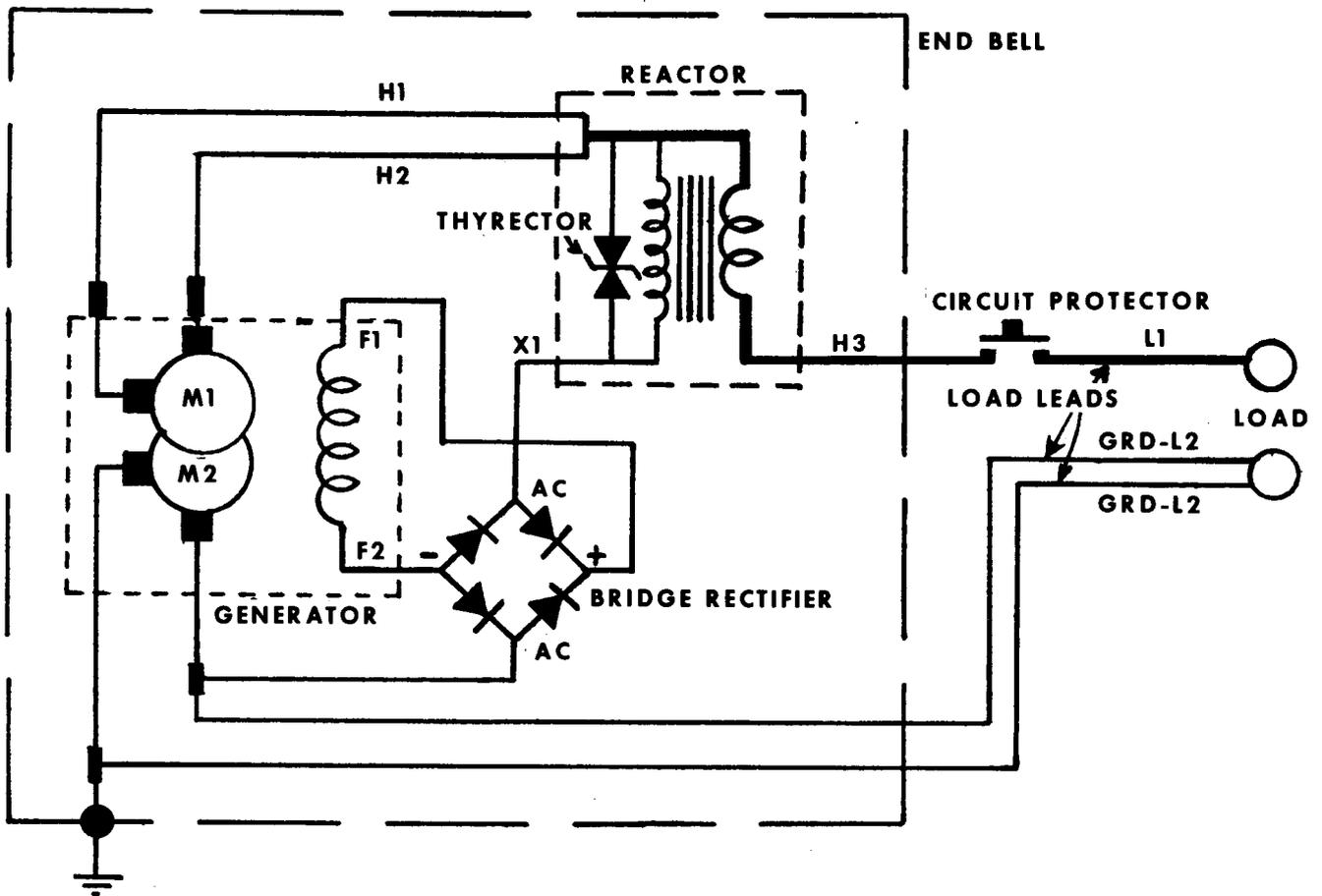
FIGURE 57. AC GENERATOR SCHEMATIC
