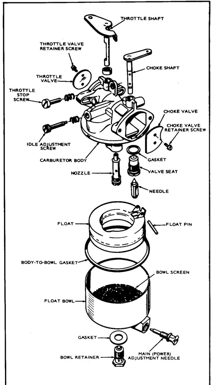
FIGURE 29. EXPLODED VIEW OF CARBURETOR
