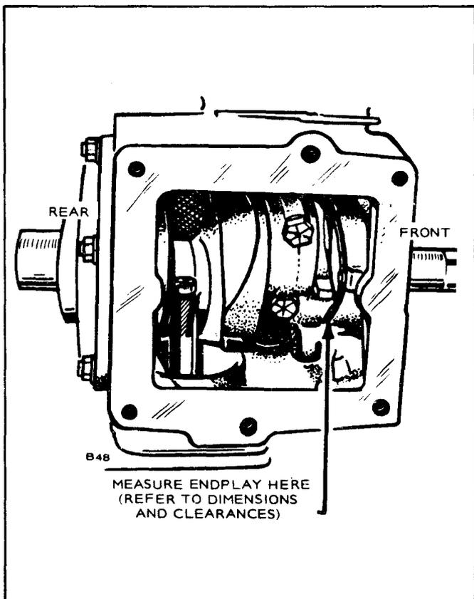
FIGURE 18. CRANKSHAFT ENDPLAY
