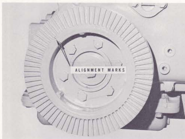
Fig. 3-14. Vibration damper alignment marks
