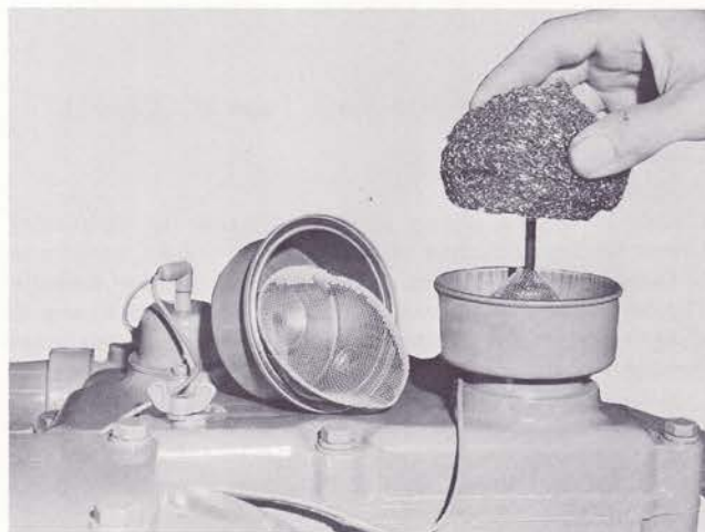
Fig. 3-12. Installing clean wire-mesh element
