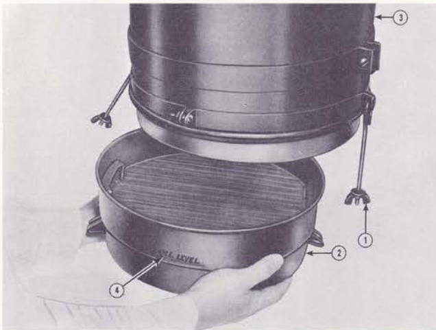
Fig. 3-9. Checking air cleaner oil level
