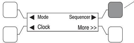
The Sequencer sub-menus are a software only feature allowing the user to send a predetermined sequence of network event announcements. The announcements are sent in a timed, sequential order and are used to turn ATS loads off and on.
