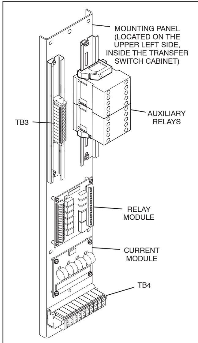
FIGURE 2-25. CONTROL WIRING CONNECTIONS
