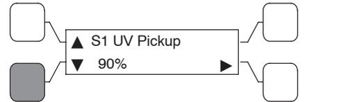
Under-Voltage Sensor Drop-Out Voltage
