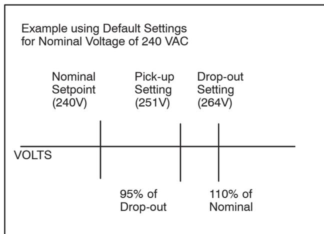
FIGURE 3-14. OVER-VOLTAGE SENSING
