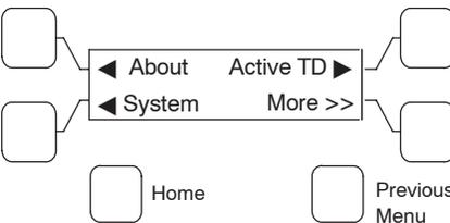
The ACTIVE TD button displays all active time delays.
