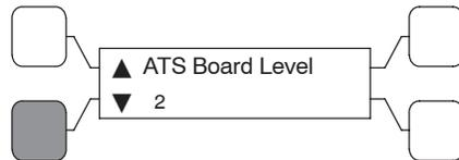
This screen indicates if a Network Communications Module is installed and enabled.
