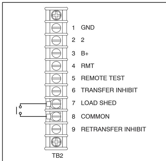
**FIGURE 2-24. TB2 CONNECTIONS FOR LOAD SHED OPTION**
