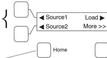
The LOAD key moves through sub-menus to display information on the Load connected source:
