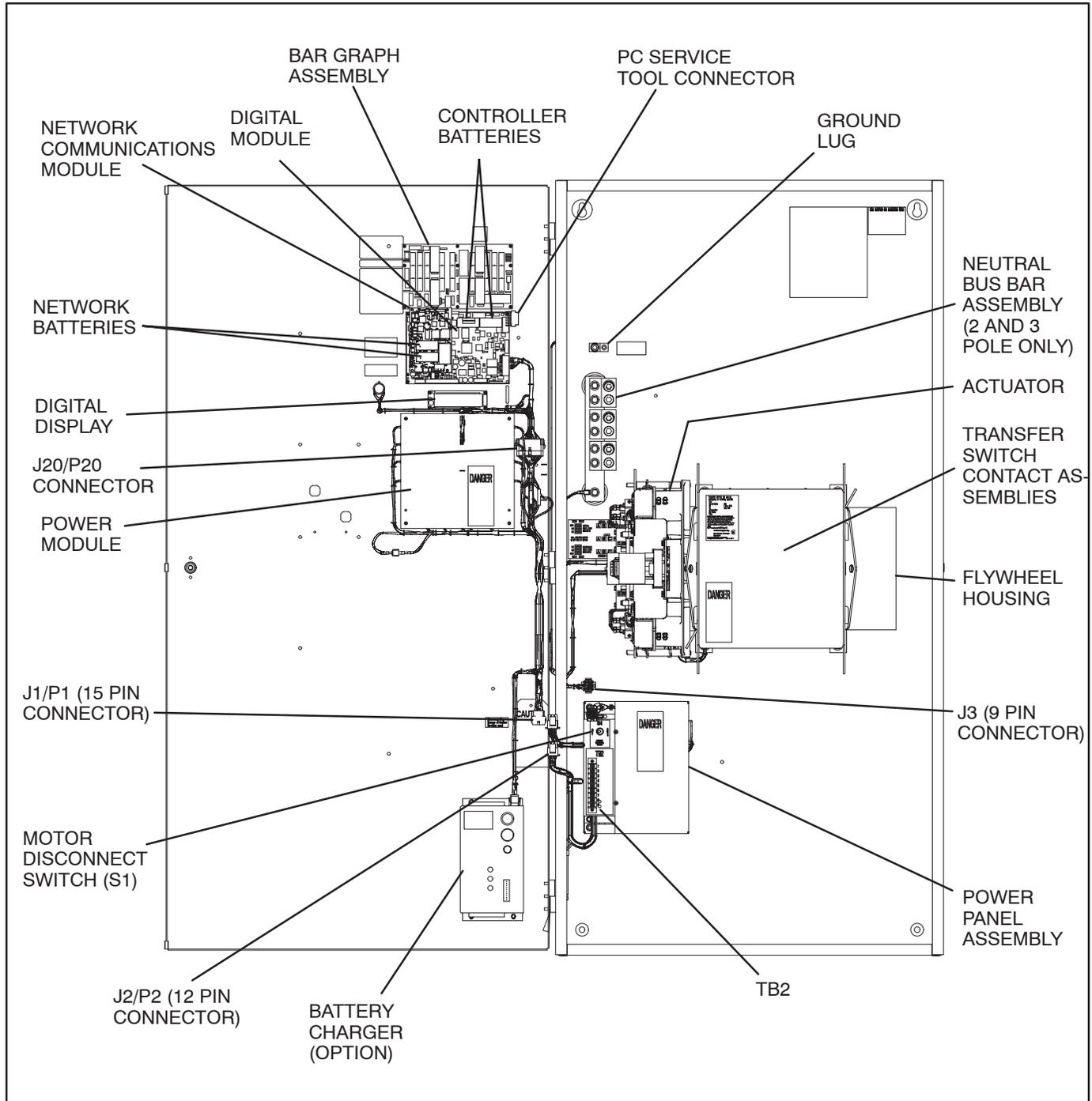
FIGURE 2-12. INTERIOR COMPONENTS (300-600 AMP SWITCH SHOWN)
