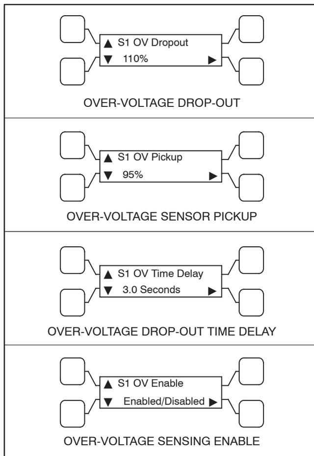
FIGURE 3-15. OVER-VOLTAGE SENSING SUB-MENUS
