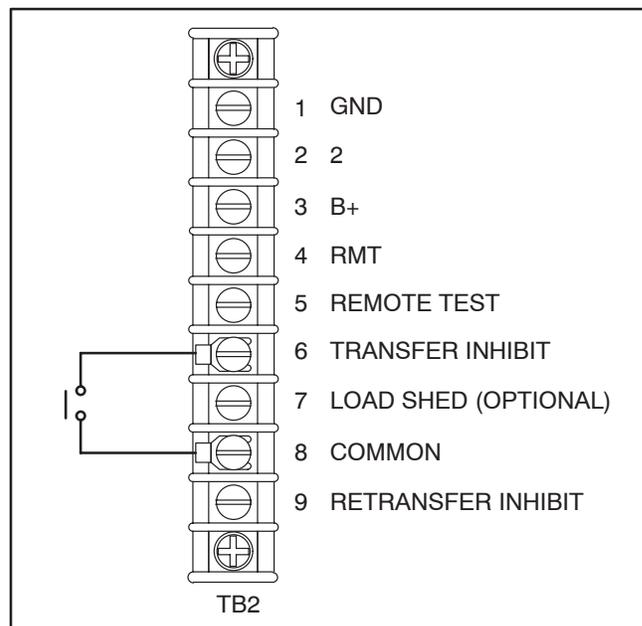
FIGURE 2-9. TB2 CONNECTIONS FOR TRANSFER INHIBIT
