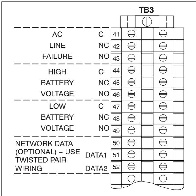
**FIGURE 2-23. BATTERY CHARGER ALARM CONTACTS AND NETWORK CONNECTIONS**
