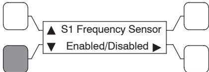
Monitors line frequency on A-Phases of both sources (Enabled).
