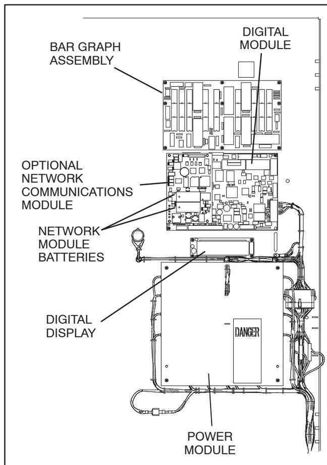
FIGURE 2-8. INTERIOR CONTROL COMPONENTS
