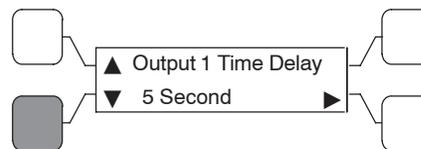
If the Sequence Length is greater than 1, the control counts down the specified Relay 2 time delay, then activates the Relay 2 signal.
