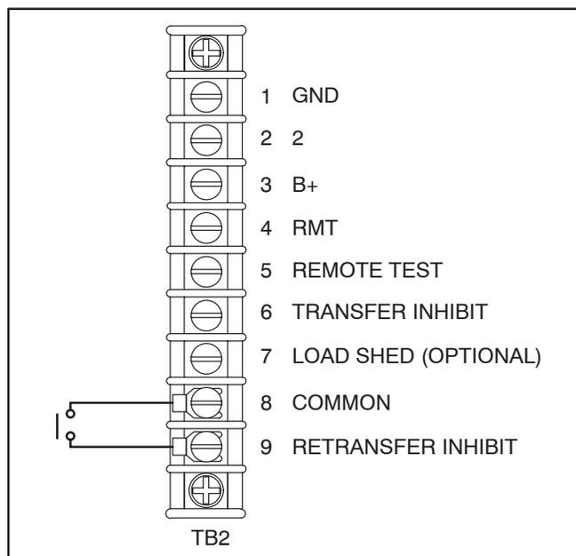
**FIGURE 2-10. TB2 CONNECTIONS FOR RETRANSFER INHIBIT**
