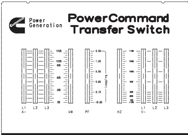
FIGURE 2-2. BAR GRAPH METER PANEL
