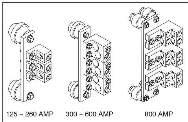
**FIGURE 2-16. NEUTRAL BAR ASSEMBLIES FOR 2-POLE AND 3-POLE TRANSFER SWITCHES**
