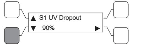
Under-Voltage Drop-Out Time Delay
