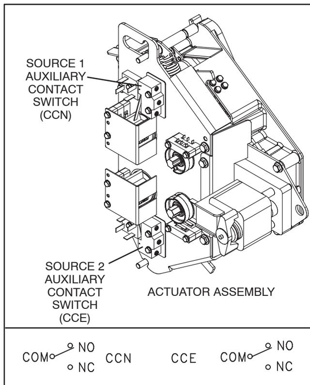
**FIGURE 2-17. AUXILIARY CONTACT SWITCHES**
