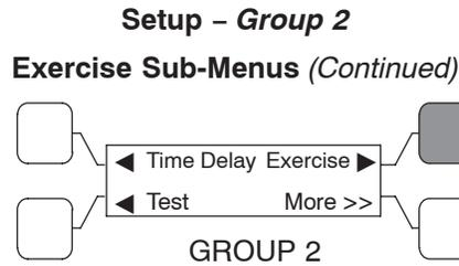
Level 2 Controllers allow for two exercise programs to be setup from the Setup menu screen. Six additional programs and eight exceptions can be setup using the PC Service tool.
