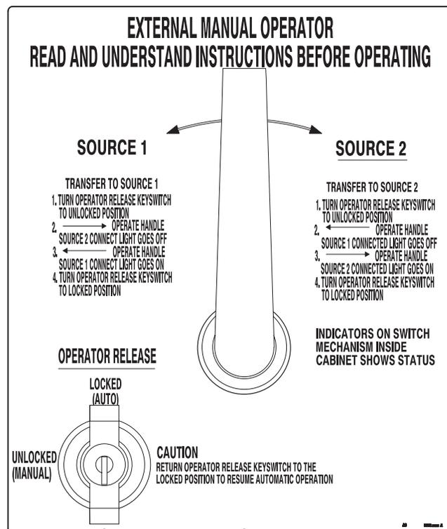
FIGURE 3-31. MANUAL OPERATOR HANDLE
