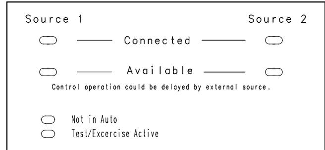
FIGURE 2-3. SWITCH PANEL INDICATOR LAMPS
