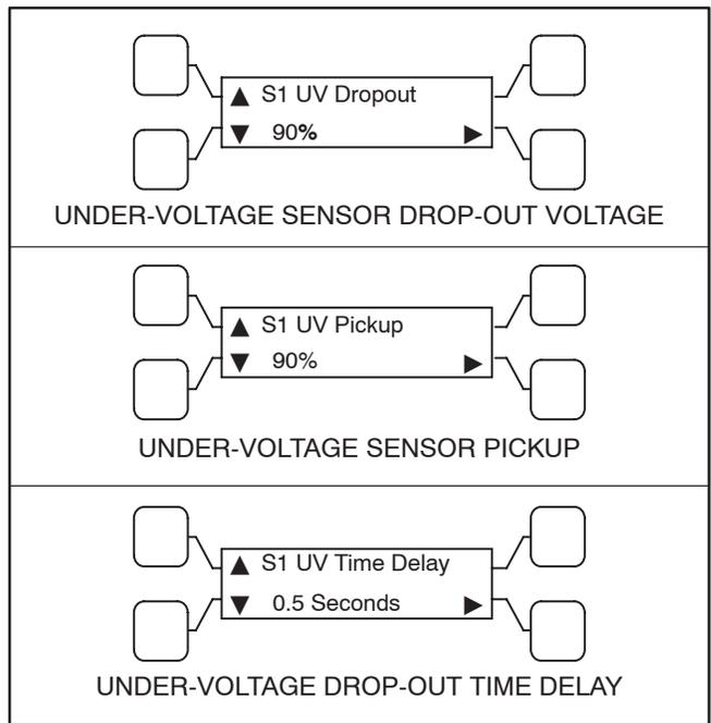
**FIGURE 3-13. UNDER-VOLTAGE SENSING SUB-MENUS**
