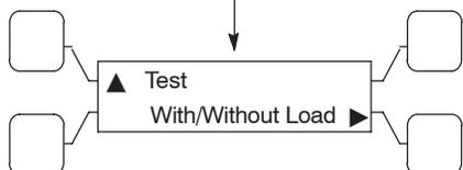
Allows an operator to automatically test the transfer switch, generator and power system.
