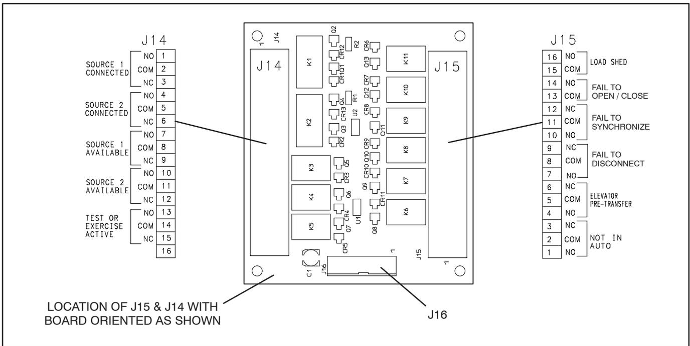
FIGURE 2-26. OPTIONAL RELAY MODULE
