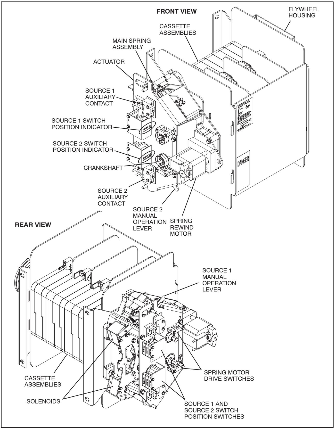
**FIGURE 2-13. ACTUATOR AND TRANSFER SWITCH (300-600 AMP SWITCH SHOWN)**
