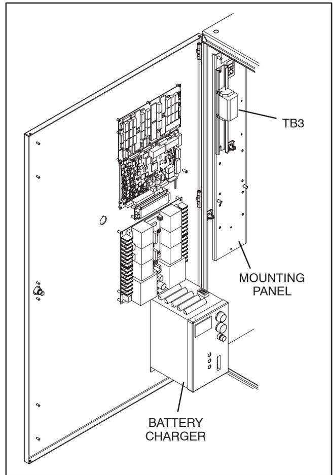
FIGURE 2-22. 10-AMPERE BATTERY CHARGER WITH BATTERY CHARGER ALARM CONTACTS
