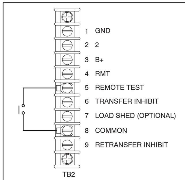
**FIGURE 2-11. TB2 CONNECTIONS FOR REMOTE TEST TRANSFER**
