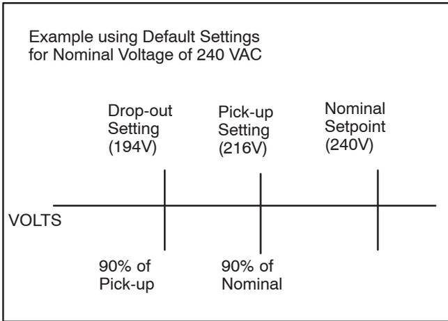
**FIGURE 3-12. UNDER-VOLTAGE SENSING**
