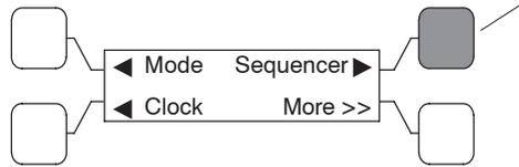
The Sequencer sub-menus are a software only feature allowing the user to send a predetermined sequence of network event announcements. The announcements are sent in a timed, sequential order and are used to turn ATS loads off and on. When used, a few seconds should be allowed between load steps to allow the generator voltage and frequency to stabilize.
