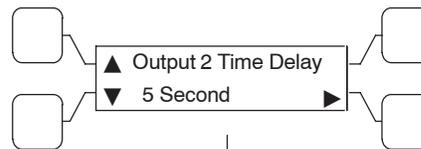
The process repeats until all relay signals have been sequenced. The maximum time delay for all 8 signals is 8 minutes.
