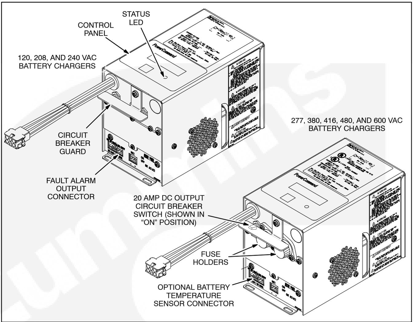
**FIGURE 2-48. 15/12-AMP POWERCOMMAND BATTERY CHARGERS**
