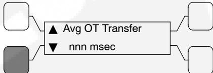
Average time over the last four transfers between the start of the command to move the switch from the old source (OT) and the position sensor sensing that the movement was completed.
