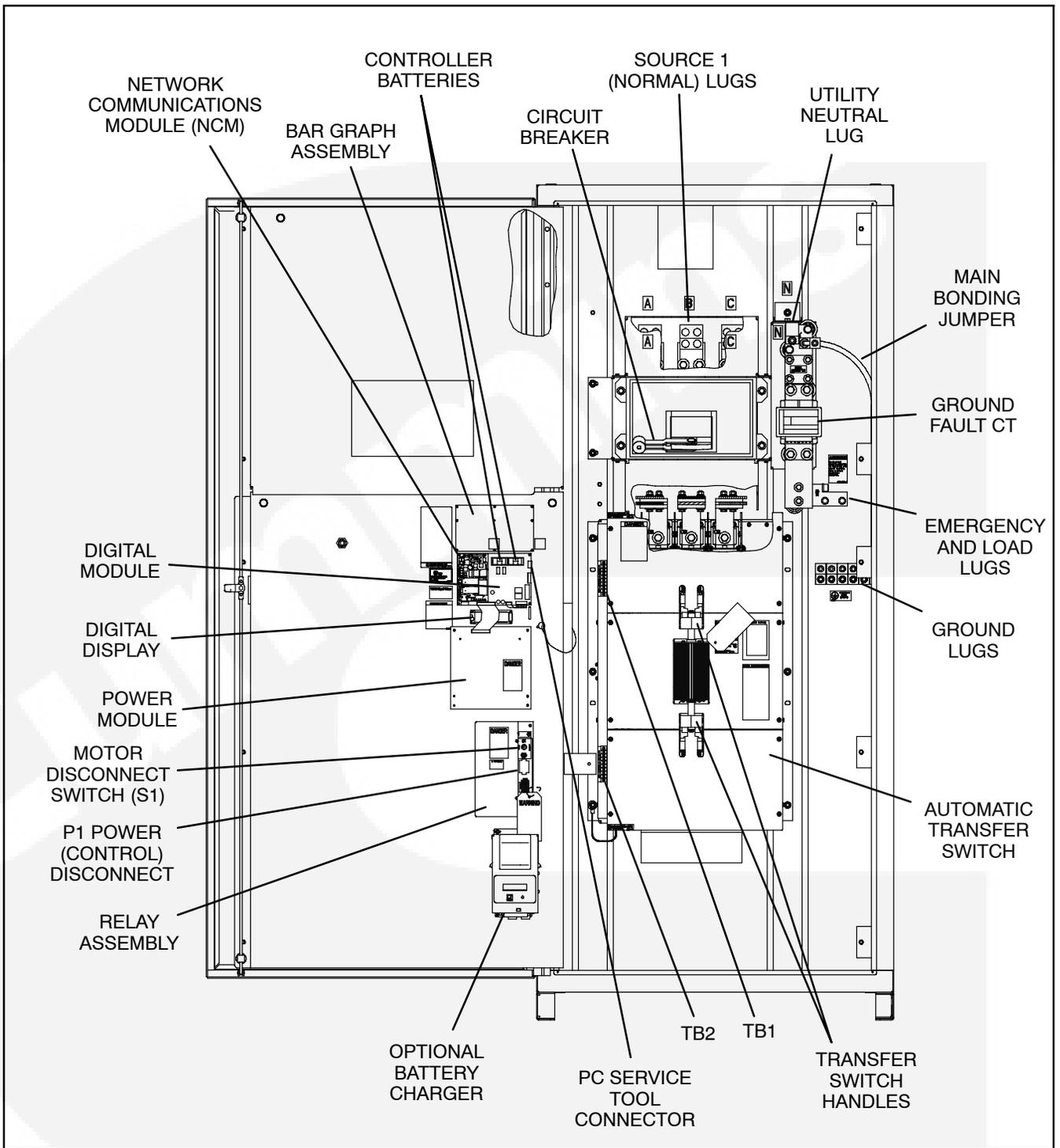
**FIGURE 2-42. INTERIOR/COMPONENTS (1000 AMP, 4 POLE, TYPE 3R AND 12 CABINET)**
