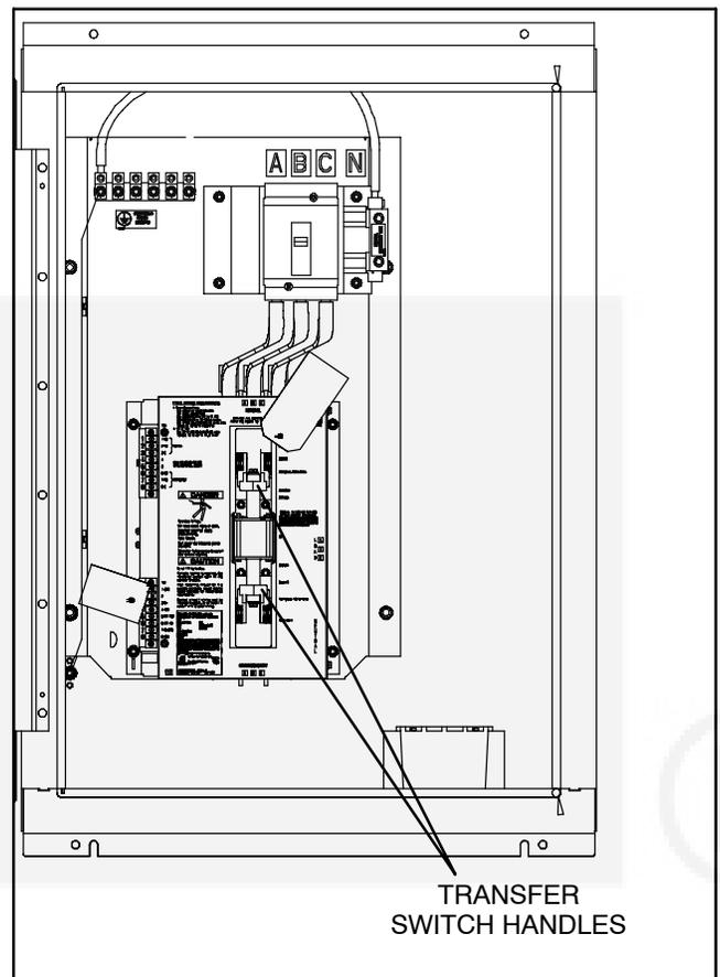
FIGURE 3-1. MANUAL OPERATION, 40-1000 AMP SWITCHES
