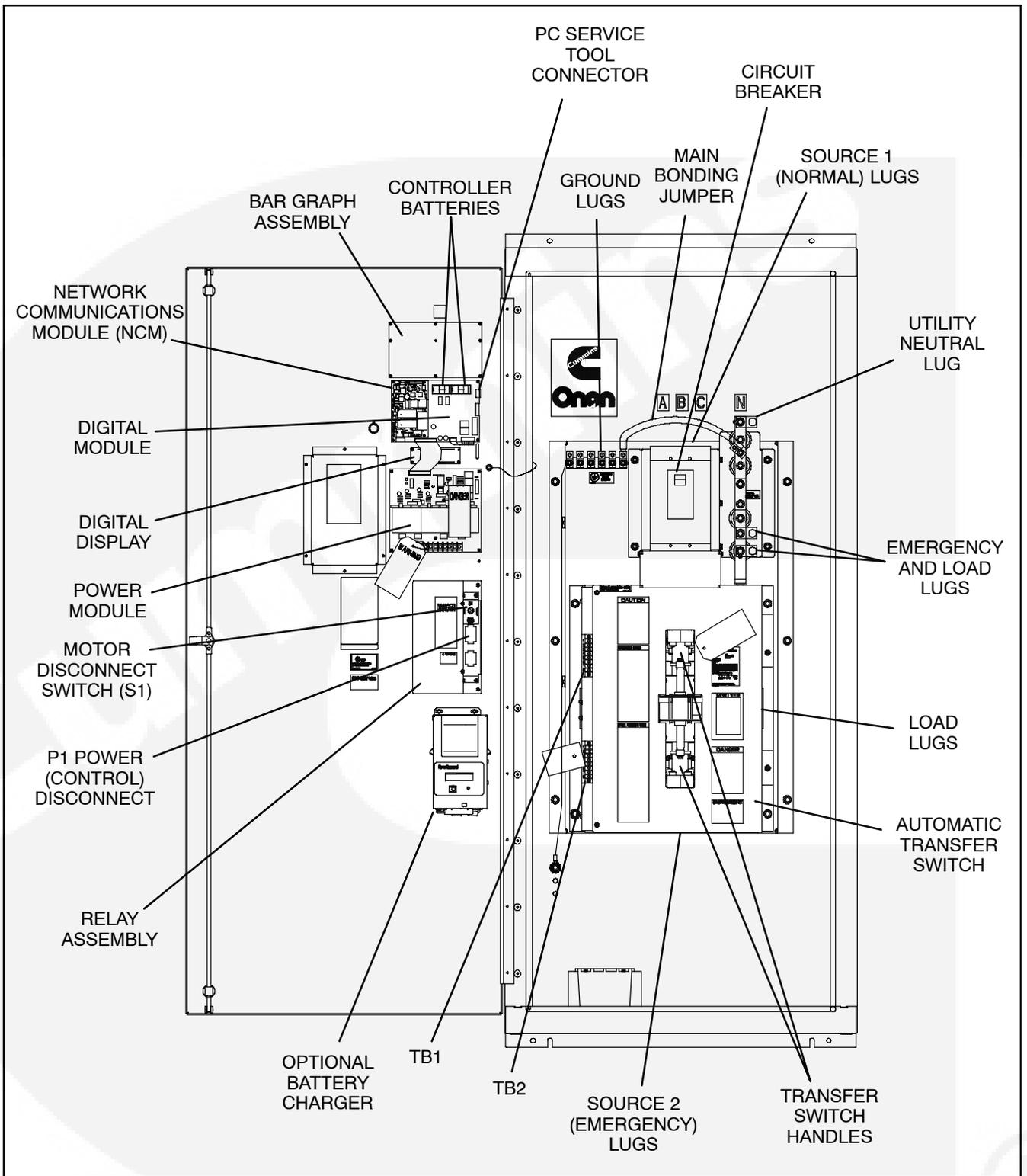
FIGURE 2-40. INTERIOR/COMPONENTS (150-250 AMP, 3 POLE, TYPE 1 CABINET)
