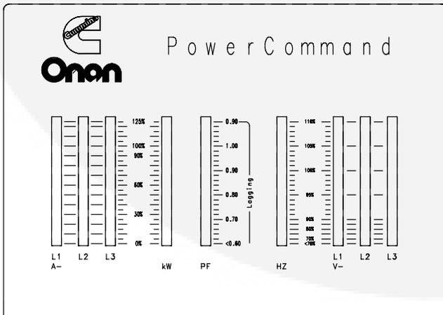
FIGURE 2-2. BAR GRAPH METER PANEL
