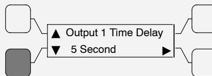
If the Sequence Length is greater than 1, the control counts down the specified Relay 2 time delay, then activates the Relay 2 signal.
