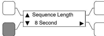
When Load Sequencer is triggered, the controller deactivates all remote relay output signals. Starting with Relay 1, the controller counts down the specified time delay, then activates Relay 1.
