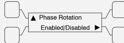
The phase rotation sensing can be enabled or disabled (Enabled).
