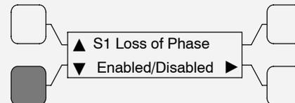
The loss of single phase sensing can be enabled or disabled (Disabled).
