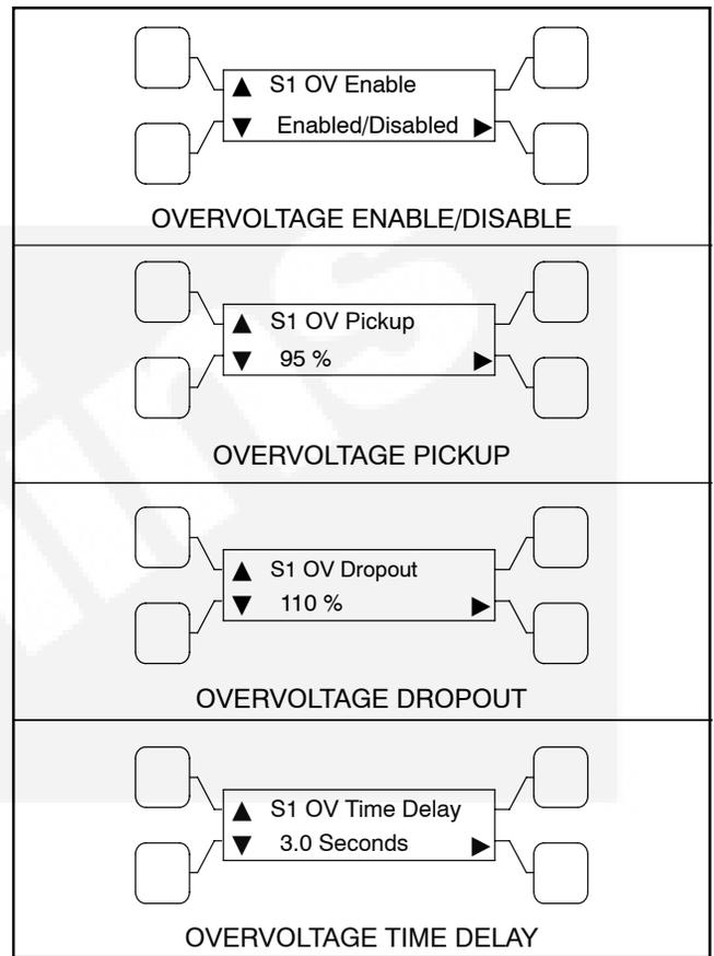
**FIGURE 2-16. OVER-VOLTAGE SENSING SUBMENUS**
