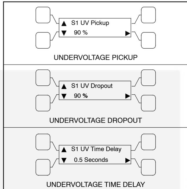
FIGURE 2-14. UNDER-VOLTAGE SENSING SUBMENUS
