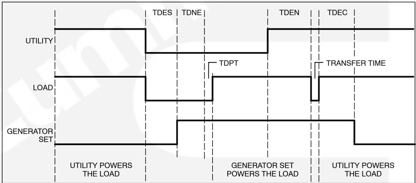
**FIGURE 2-23. OPEN TRANSITION WITH SYNC CHECK**
