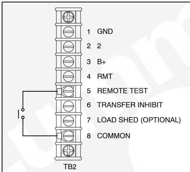
**FIGURE 2-30. TB2 CONNECTIONS FOR REMOTE TEST TRANSFER**
