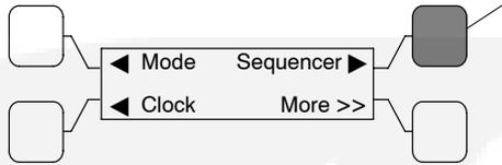
The Sequencer submenus are a software only feature allowing the user to send a predetermined sequence of network event announcements. The announcements are sent in a timed, sequential order and are used to turn ATS loads off and on. When used, a few seconds should be allowed between load steps to allow the generator voltage and frequency to stabilize.
