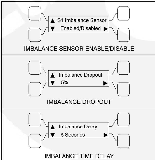
**FIGURE 2-19. VOLTAGE IMBALANCE SENSOR SUBMENUS**
