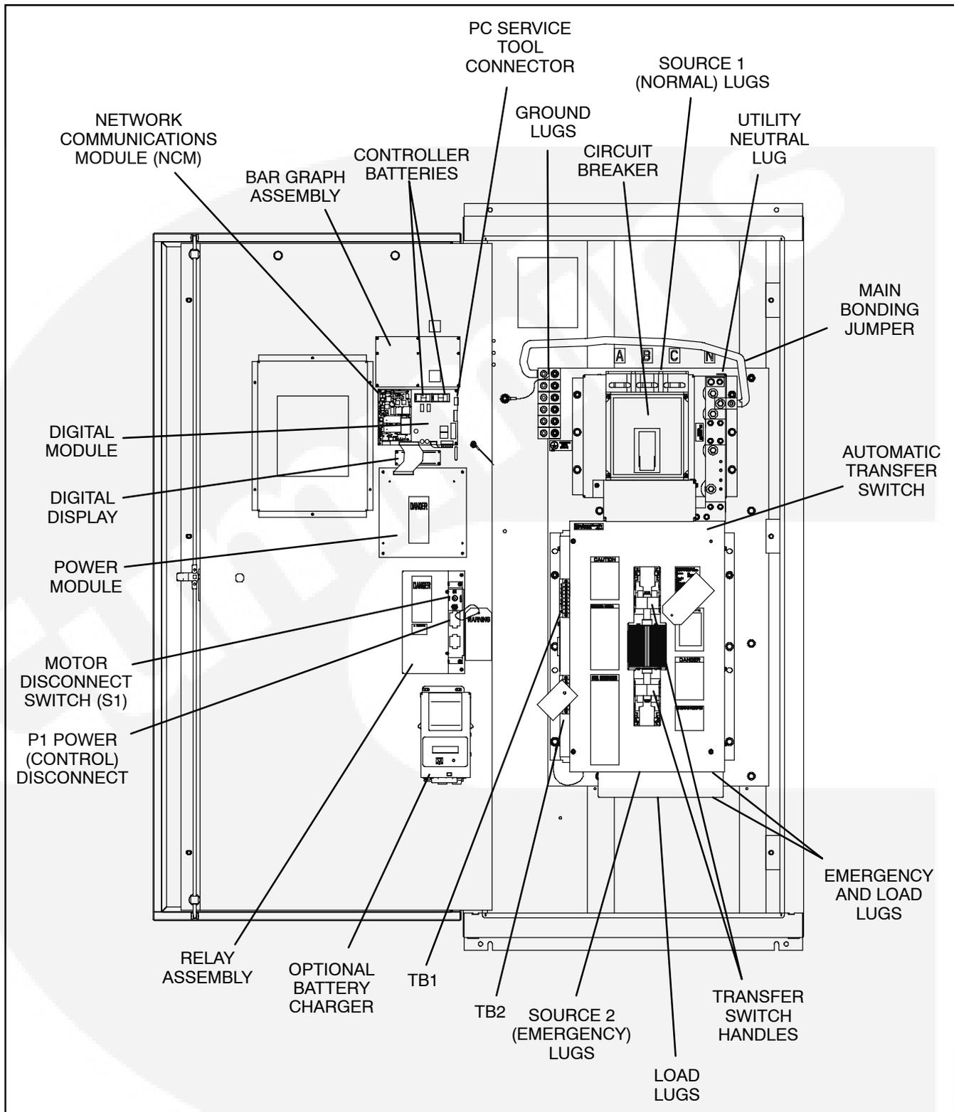
**FIGURE 2-41. INTERIOR/COMPONENTS (300-600 AMP, 4 POLE, TYPE 3R AND 12 CABINET)**
