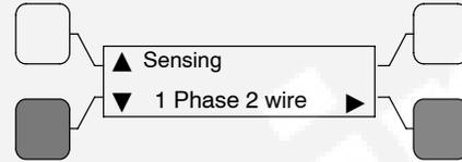
Delta or Wye Configuration. This menu is only displayed with Level 2 Controllers.
