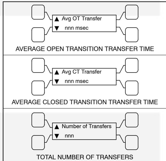
**FIGURE 2-33. TRANSFER SUBMENUS**
