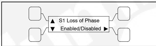
FIGURE 2-21. LOSS OF PHASE SENSING SUBMENU
