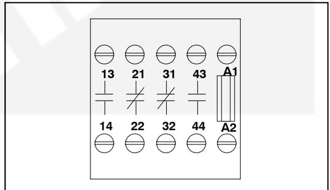
**FIGURE 2-50. AUXILIARY RELAY TERMINALS**
