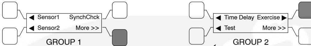
Level 1 Controllers allow for setting two exercise periods and Level 2 Controllers allow for setting eight exercise periods from the digital display screen.
