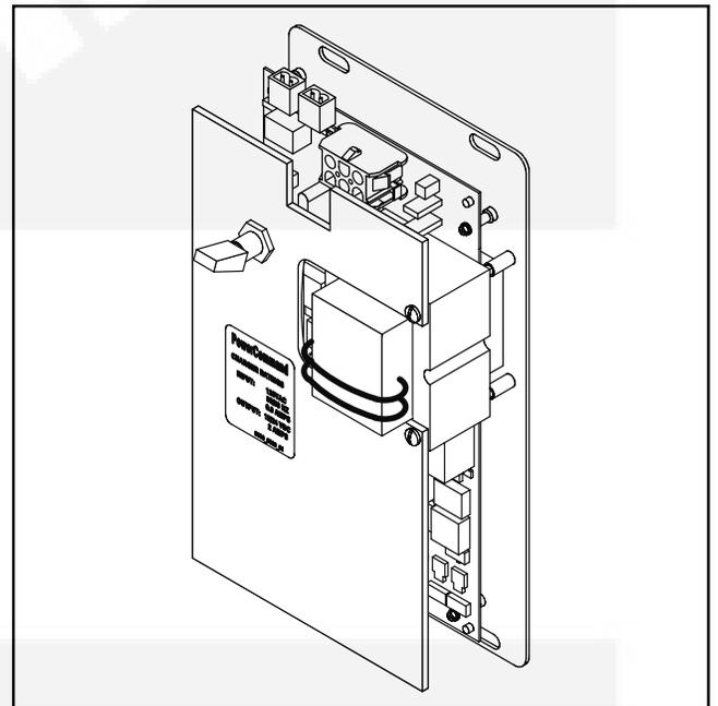
**FIGURE 2-45. 2-AMP POWERCOMMAND BATTERY CHARGER**
