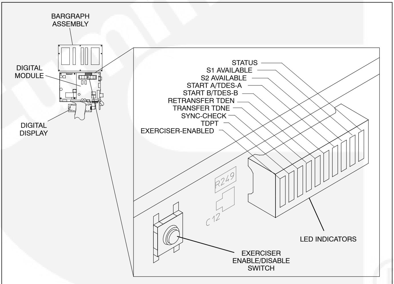
FIGURE 6-1. LED LOCATION ON DIGITAL MODULE
