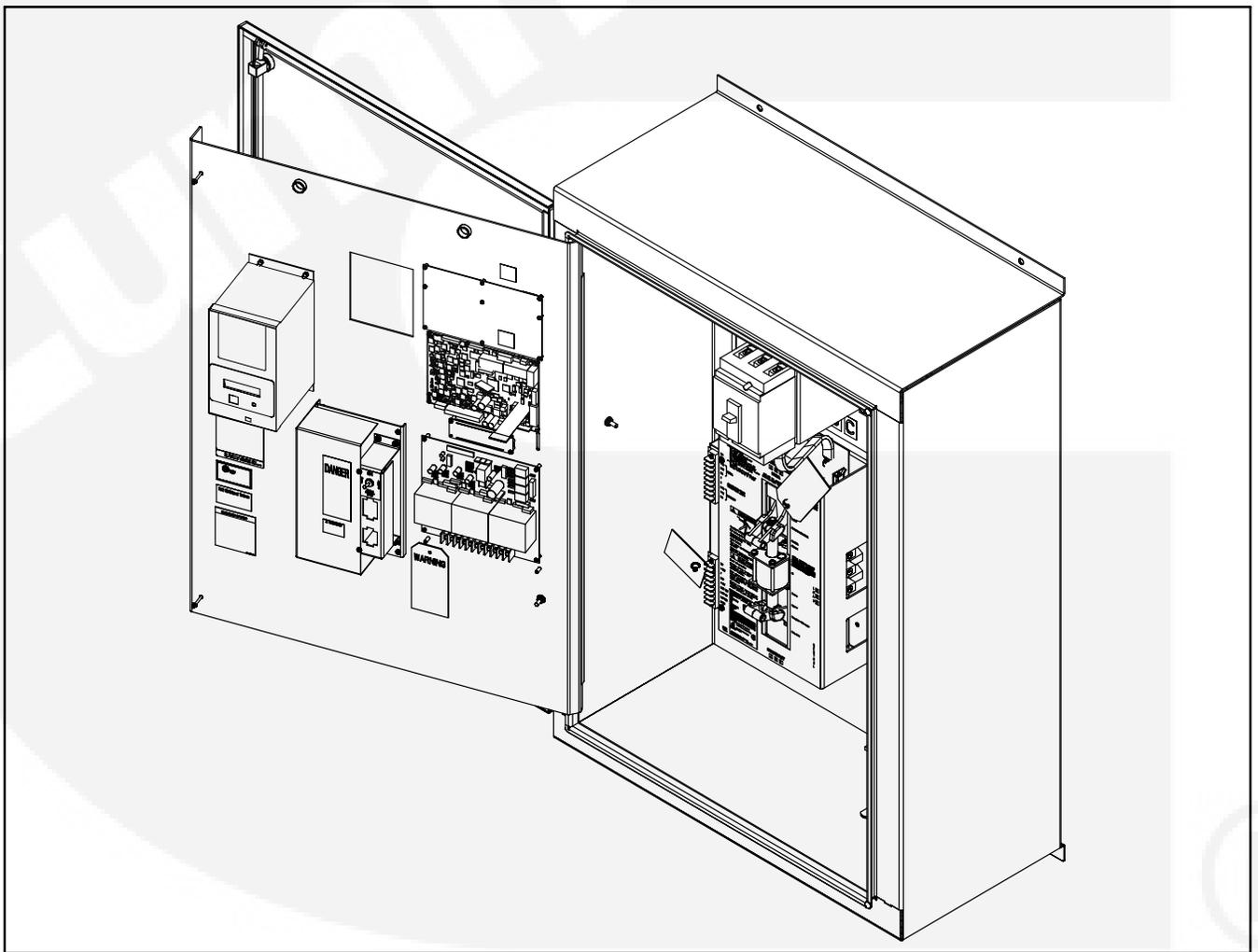
FIGURE 1-1. OTPC SERVICE ENTRANCE TRANSFER SWITCH (40-125 AMP, TYPE 3R AND 12 CABINET SHOWN)
