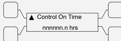
Displays the amount of time the controller board has been operating since initialization. Value is stored permanently.
