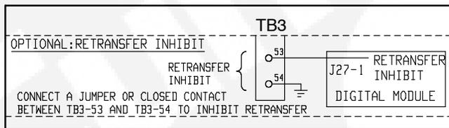
**FIGURE 2-32. TB3 CONNECTIONS FOR RETRANSFER INHIBIT**
