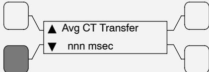
Average time over the last four transfers between the start of the command to close the new switch (CT) and the position sensor sensing that the movement was completed. NOTE: This function is not available with service entrance transfer switches.
