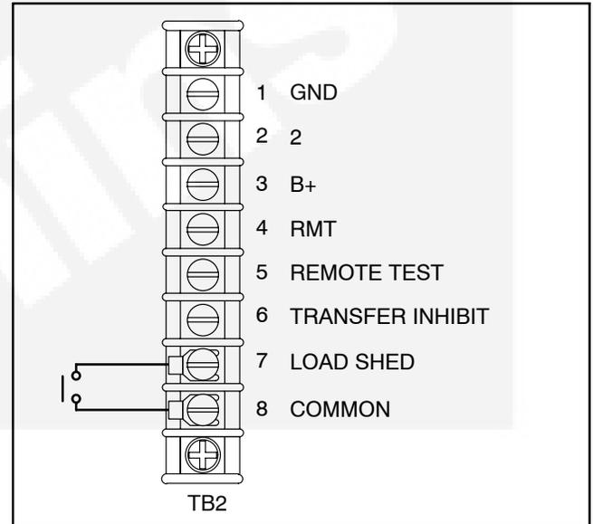
FIGURE 2-62. LOAD SHED TB2 CONNECTION
