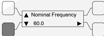
Enter a frequency between 45 and 65 Hz (60 Hz).
