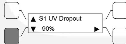
Under-Voltage Drop-Out Time Delay
