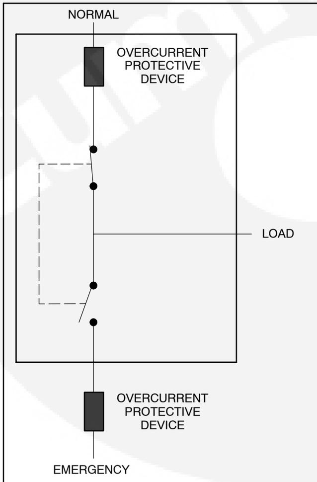
**FIGURE 1-3. LOAD TRANSFER SWITCH (TYPICAL FUNCTION)**
