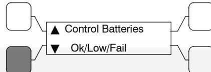
Status of lithium batteries on controller board
