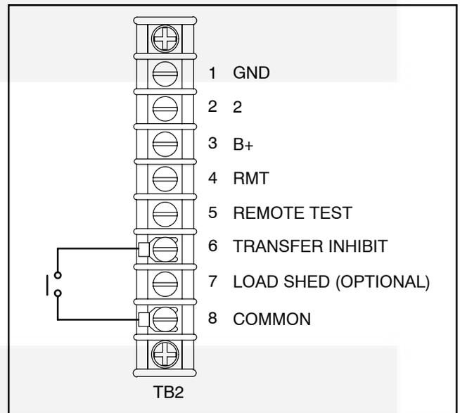
**FIGURE 2-31. TB2 CONNECTIONS FOR TRANSFER INHIBIT**
