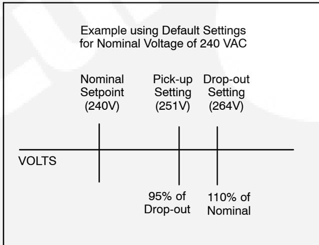
**FIGURE 2-15. OVER-VOLTAGE SENSING**
