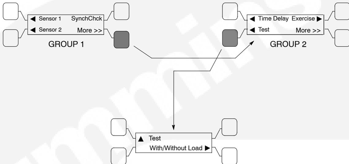
Allows an operator to automatically test the transfer switch, generator and power system.
