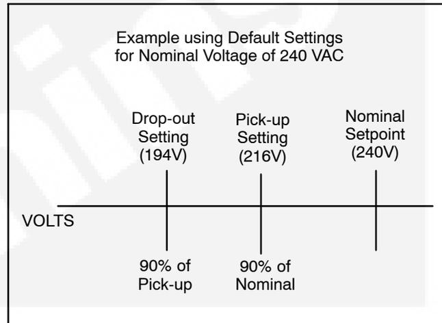
FIGURE 2-13. UNDER-VOLTAGE SENSING
