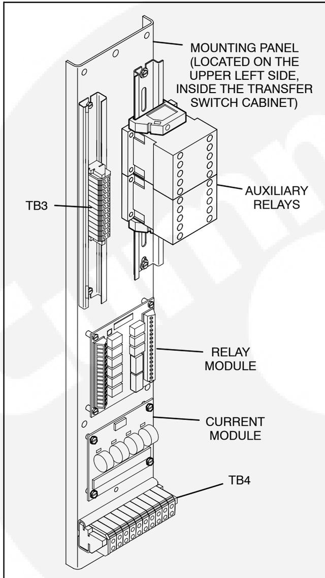
**FIGURE 2-49. CONTROL WIRING CONNECTIONS**
