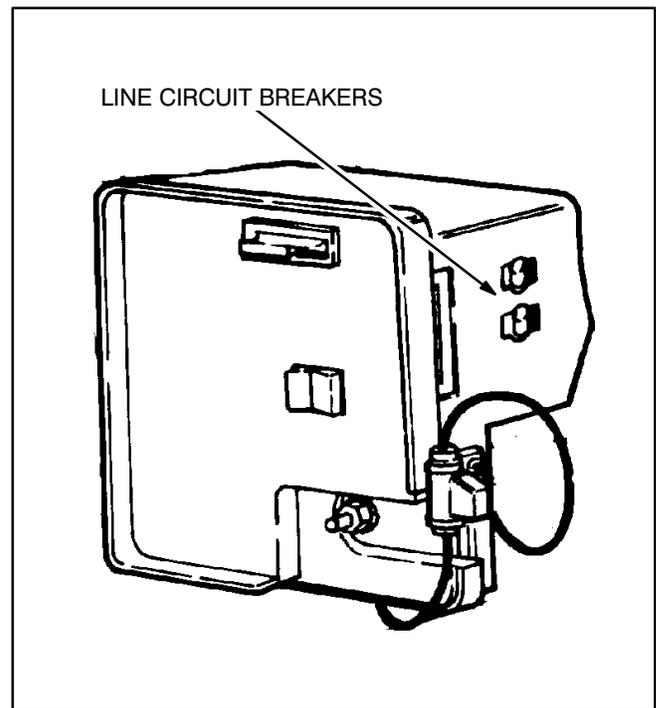
FIGURE 9. SET MOUNTED CIRCUIT BREAKER
