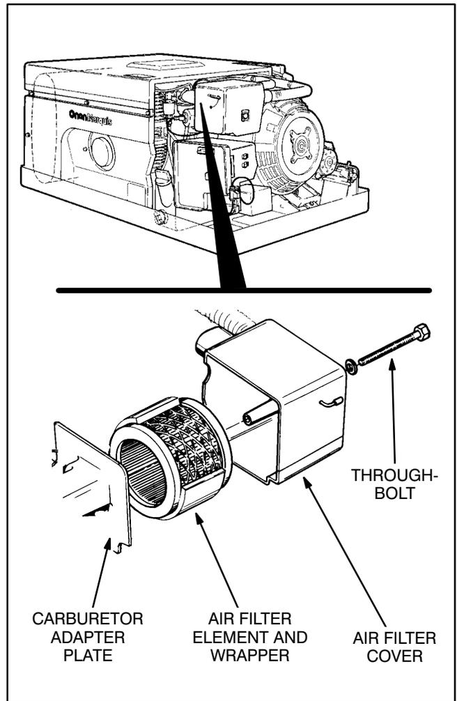
FIGURE 15. AIR FILTER ELEMENT AND WRAPPER
