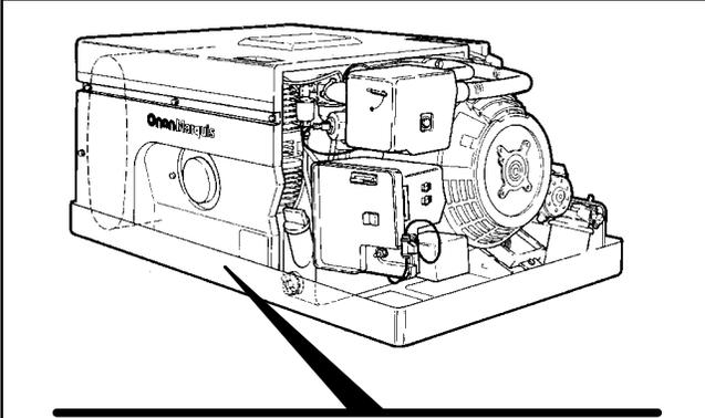
NAMEPLATE WITH TYPICAL MODEL AND SERIAL NUMBER DATA
