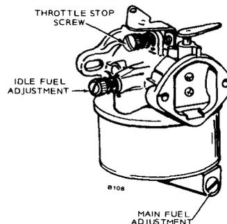
FIGURE 15. CARBURETOR ADJUSTMENTS
