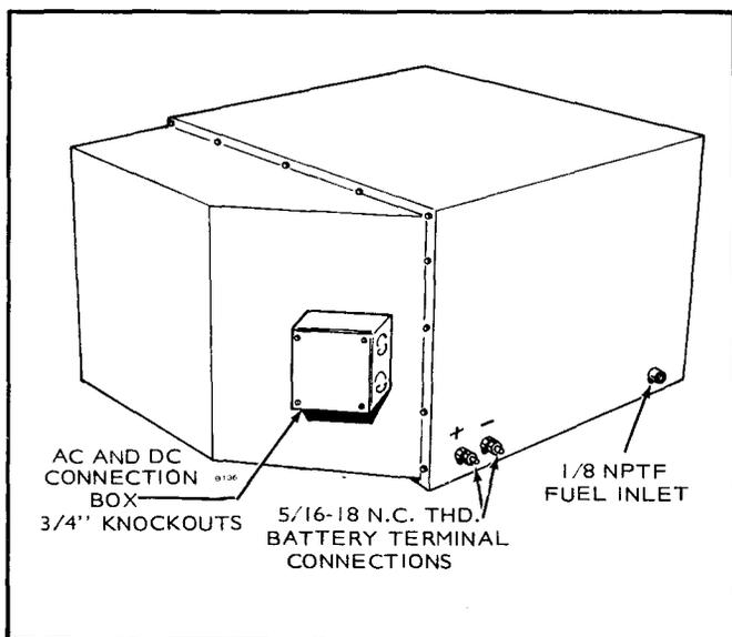
FIGURE 2. EXTERNAL CONNECTIONS
