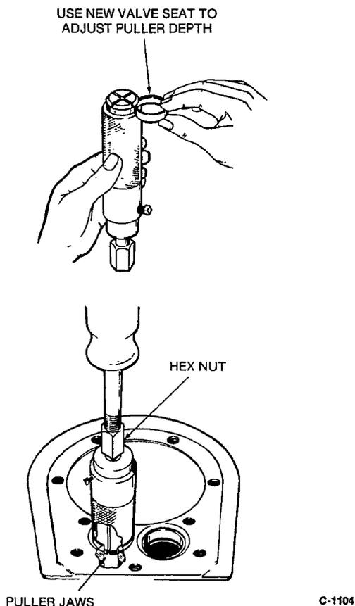
FIGURE 4. VALVE SEAT REMOVAL
