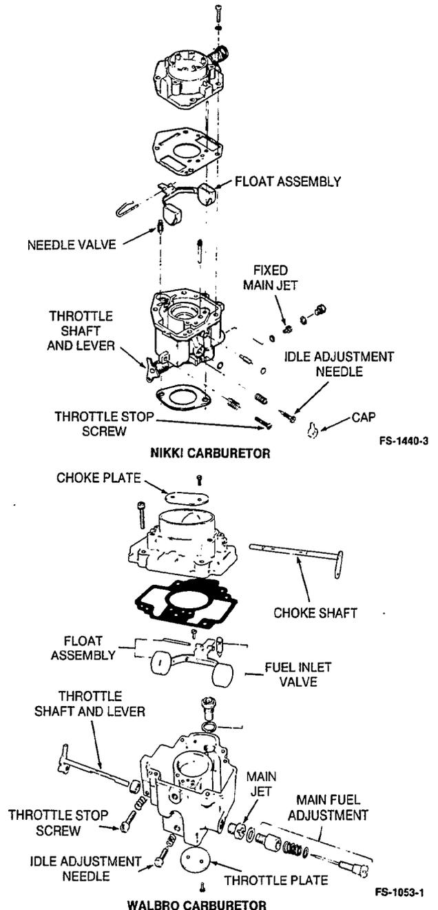
FIGURE 3. CARBURETOR ASSEMBLY
