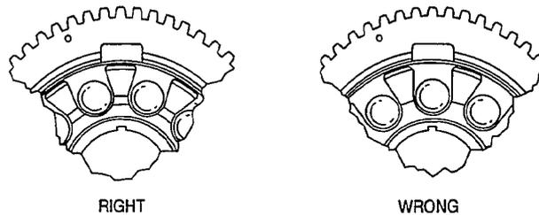
INSTALLATION OF BALL SPACER
