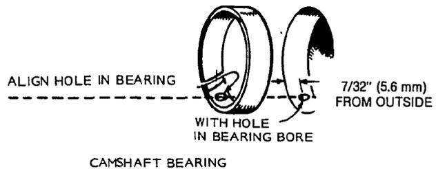
FIGURE 20. FRONT CAMSHAFT BEARING
