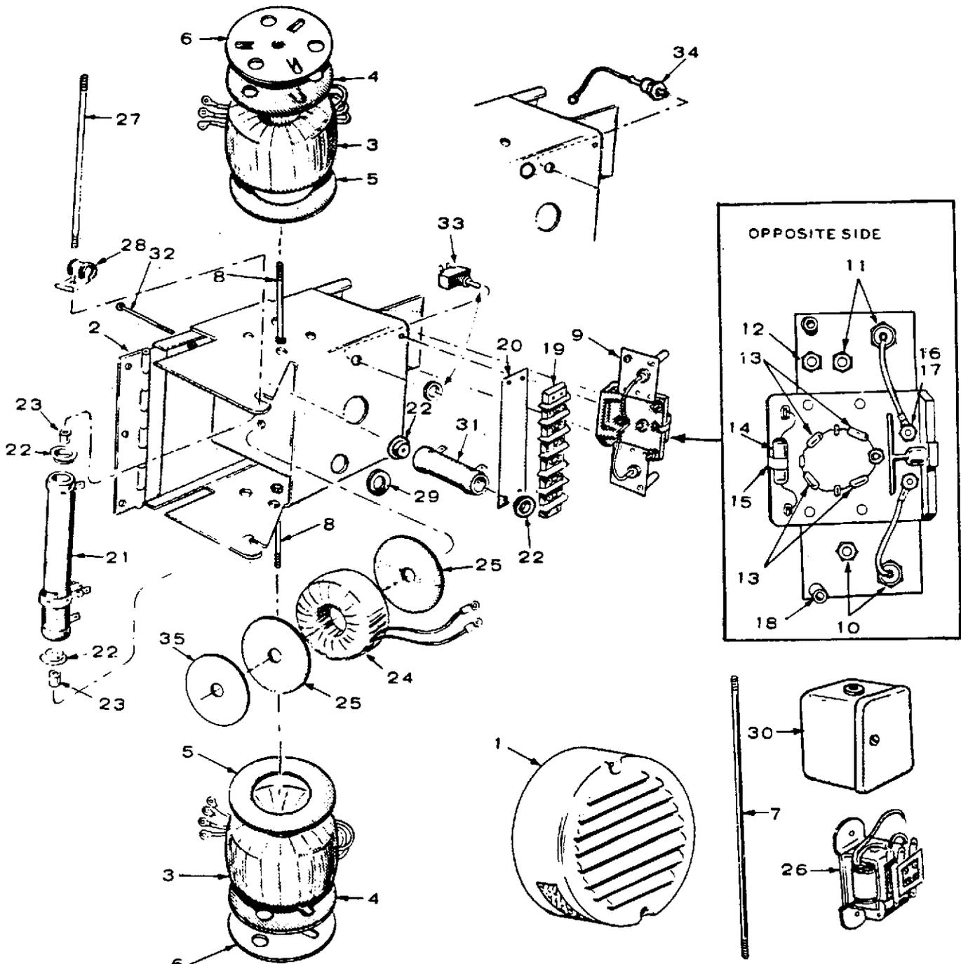
**NOTE:** 06SX1N1B used on 60 hertz Models Spec A, B & C.
