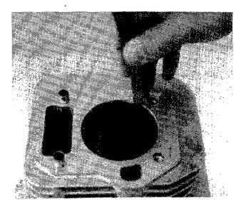
FIGURE 9-21. CHECKING RING GAP
