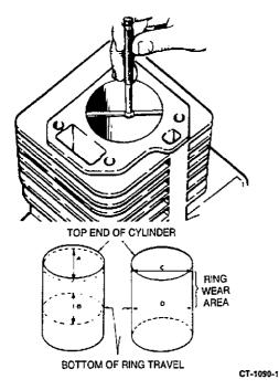
FIGURE 9-26. METHODS OF MEASURING THE DIAMETER OF A CYLINDER BORE
