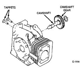
FIGURE 9-13. CAMSHAFT AND TAPPETS
