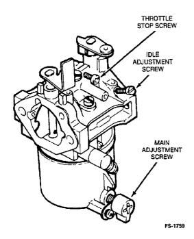
**ACAUTION** Forcing the mixture adjustment screws tight will damage the needle and seat. Turn in only until light tension can be felt.
