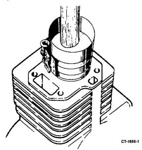
FIGURE 9-23. INSTALLING PISTON
