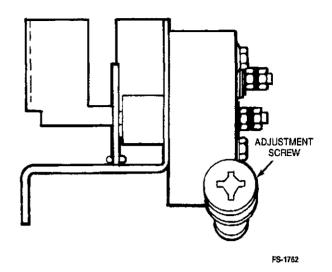
FIGURE 6-14. CHOKE ASSEMBLY
