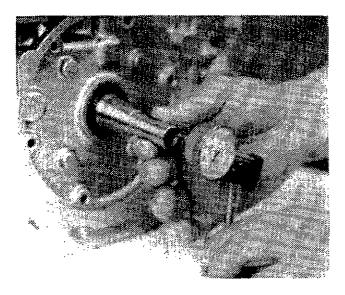
FIGURE 9-25. CHECKING ENDPLAY
