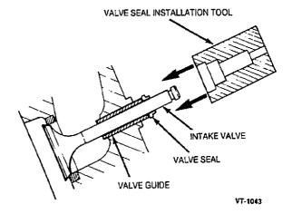
FIGURE 9-10. VALVE SEAL INSTALLATION
