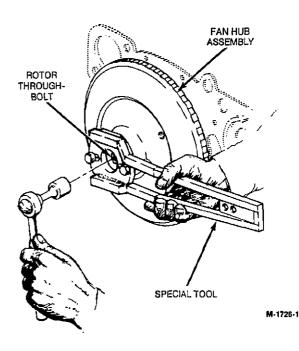
FIGURE 8-4. SECURING FAN HUB ASSEMBLY FOR REMOVAL
