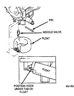
4. Invert the float and needle valve assembly and check float level by measuring between the float and carburetor at the point shown in Figure 6-13. The full weight of the float should be resting on the needle valve and spring. The correct distance is specified in Table 6-2. If the setting is incorrect, remove float and bend tab to adjust. Bend the float only at the point indicated.
