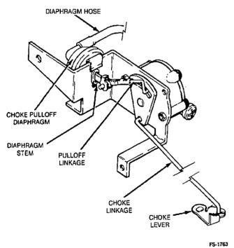
FIGURE 6-16. CHOKE PULLOFF DIAPHRAGM
