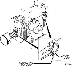
FIGURE 9-22. ROD CAP ASSEMBLY
