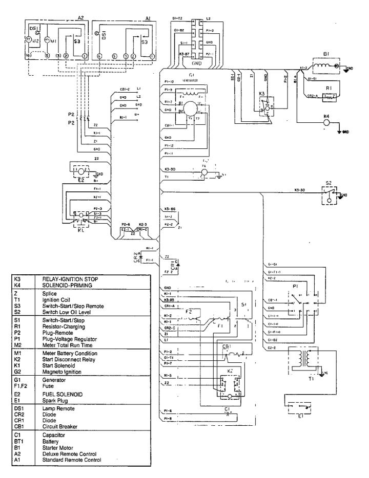
FIGURE 8-2. LPG GENERATOR SET WIRING DIAGRAM - 60 HERTZ
