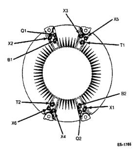
FIGURE 8-12. STATOR ASSEMBLY
