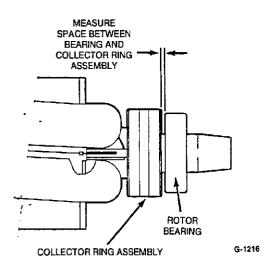
FIGURE 8-13. ROTOR BEARING SPACING
