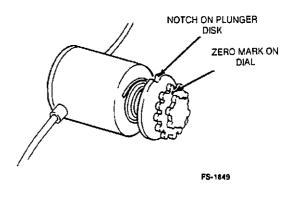
At this position there is no fuel flow when the Auto Prime is energized. To start and increase fuel flow, turn dial clockwise while manually depressing plunger.
