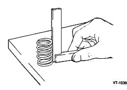
FIGURE 9-7. VALVE SPRING CHECKS
