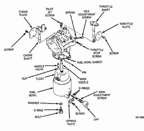
FIGURE 6-10. CARBURETOR OVERHAUL
