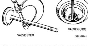
FIGURE 9-6. VALVE FACE, VALVE STEM AND VALVE GUIDE INSPECTION
