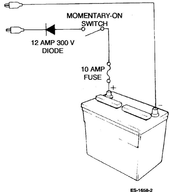
FIGURE 6-1. FIELD FLASHING CIRCUIT
