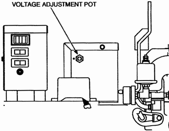
**FIGURE 6-9. LOCATION, OUTPUT VOLTAGE REGULATOR ADJUSTMENT**
