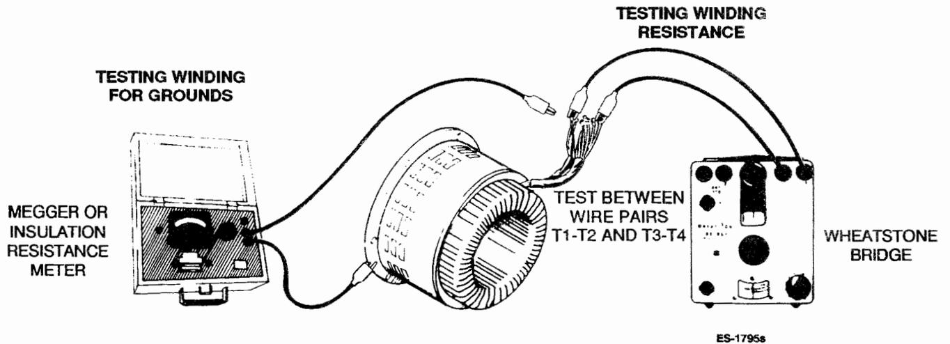
FIGURE 6-6. TESTING STATOR WINDINGS
