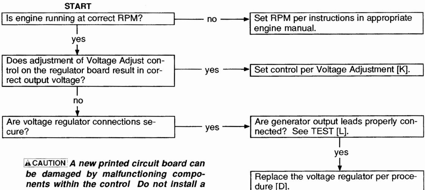
**⚠ CAUTION** A new printed circuit board can be damaged by malfunctioning components within the control. Do not install a new PC board until all other problems have been located and corrected.
