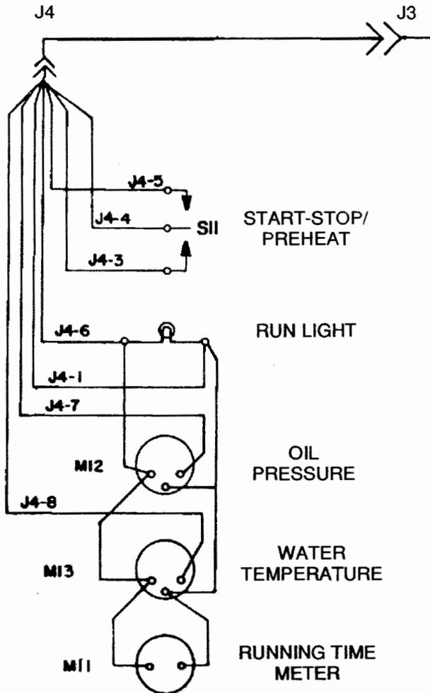
**FIGURE 2-4. REMOTE CONTROL WIRING DIAGRAM**
