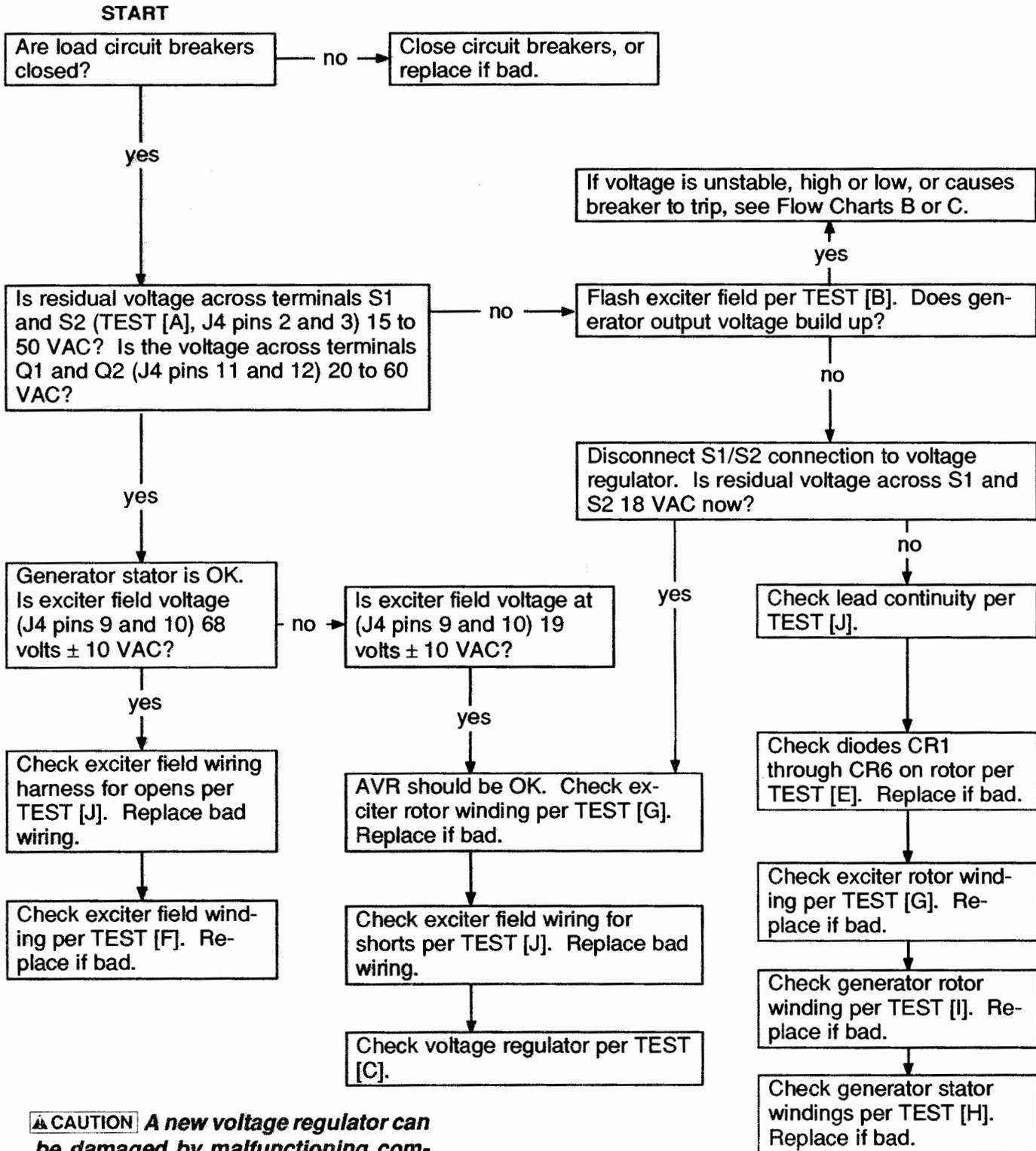
**▲CAUTION** A new voltage regulator can be damaged by malfunctioning components. Do not install a new voltage regulator until all other problems have been located and corrected.
