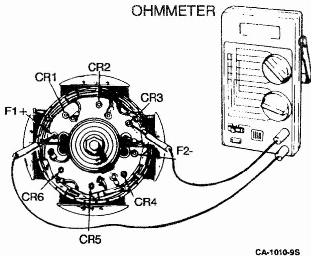
FIGURE 6-3. TESTING ROTATING RECTIFIERS
