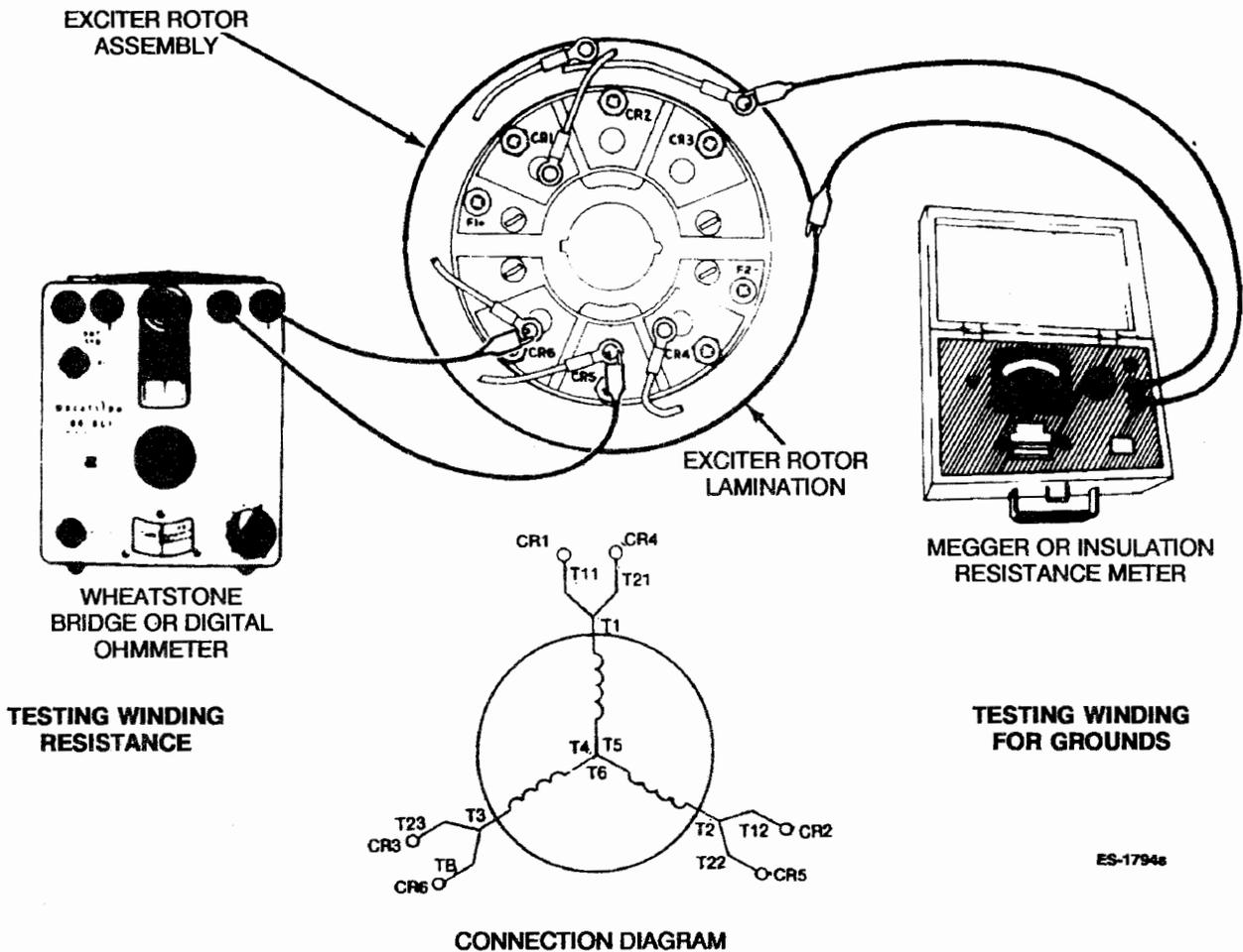
FIGURE 6-5. TESTING EXCITER ROTOR
