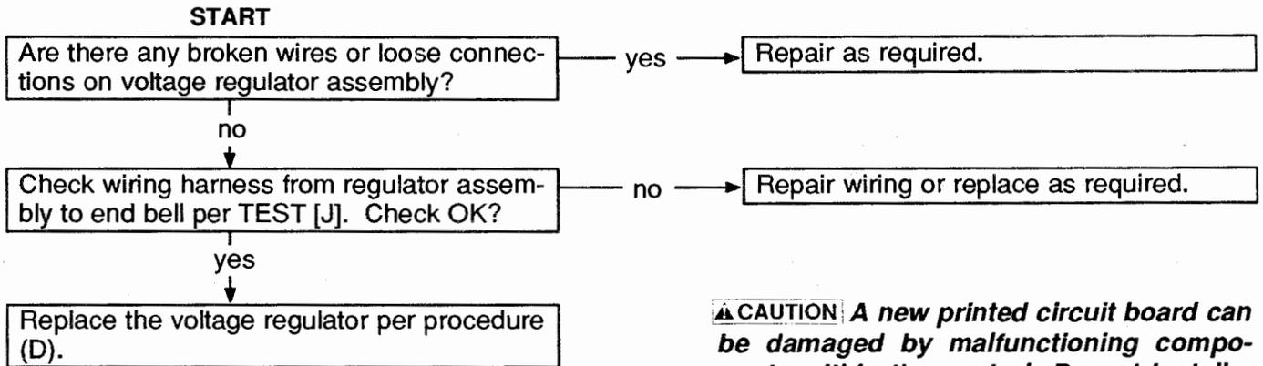
**⚠ CAUTION** A new printed circuit board can be damaged by malfunctioning components within the control. Do not install a new PC board until all other problems have been located and corrected.
