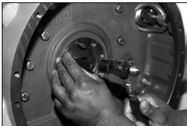
FIGURE 7-37. CENTER PUNCHING AND DRILLING EXTRACTION SCREW HOLES
