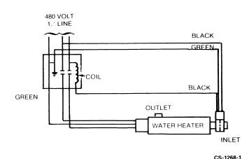
FIGURE 12. COOLANT HEATER WIRING DIAGRAMS
