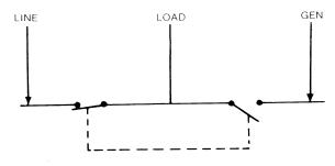
NOTE: SHOWN WITH LINE CONNECTED TO LOAD
