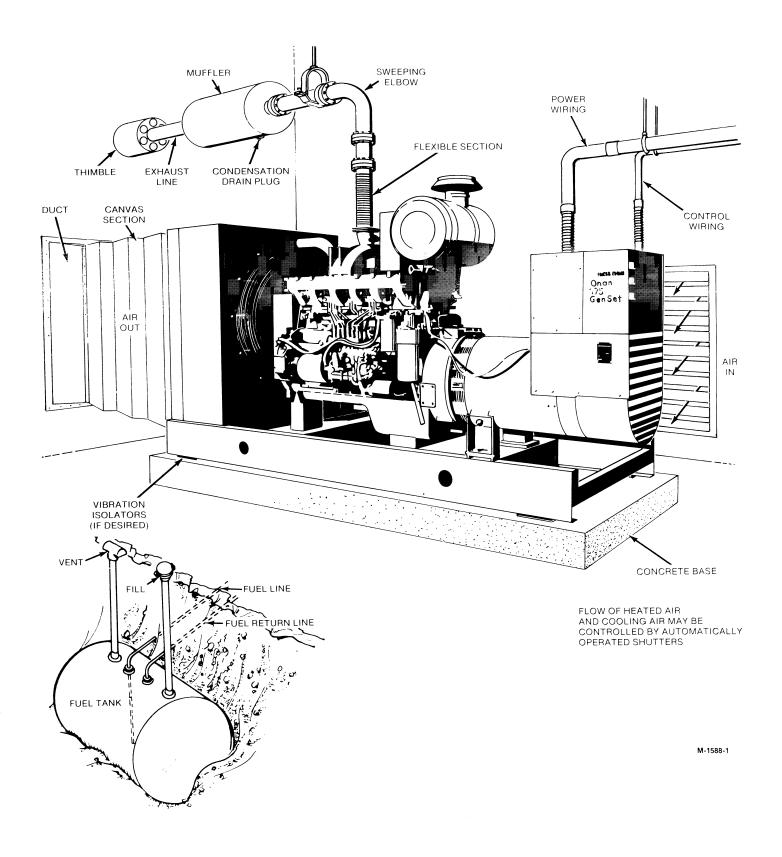
FIGURE 1. TYPICAL DV GENERATOR SET INSTALLATIONS
