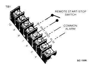
FIGURE 11. REMOTE CONTROL CONNECTIONS
