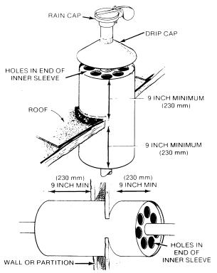
Diameter of Thimble Must Be 12 Inches (305 mm) Larger Than Diameter of Exhaust Pipe
