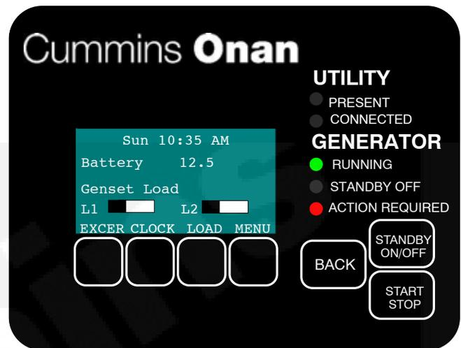
**FIGURE A-2. GENERATOR SET RUNNING—ACTION REQUIRED LAMP ON**
