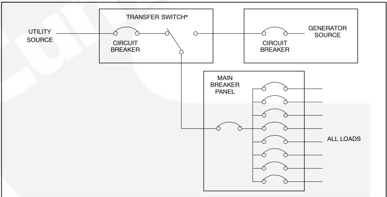
**FIGURE 4-4. FULL COVERAGE LOAD CONNECTIONS (TRANSFER SWITCH WITHOUT CONTROLLER, ONE CIRCUIT BREAKER)**
