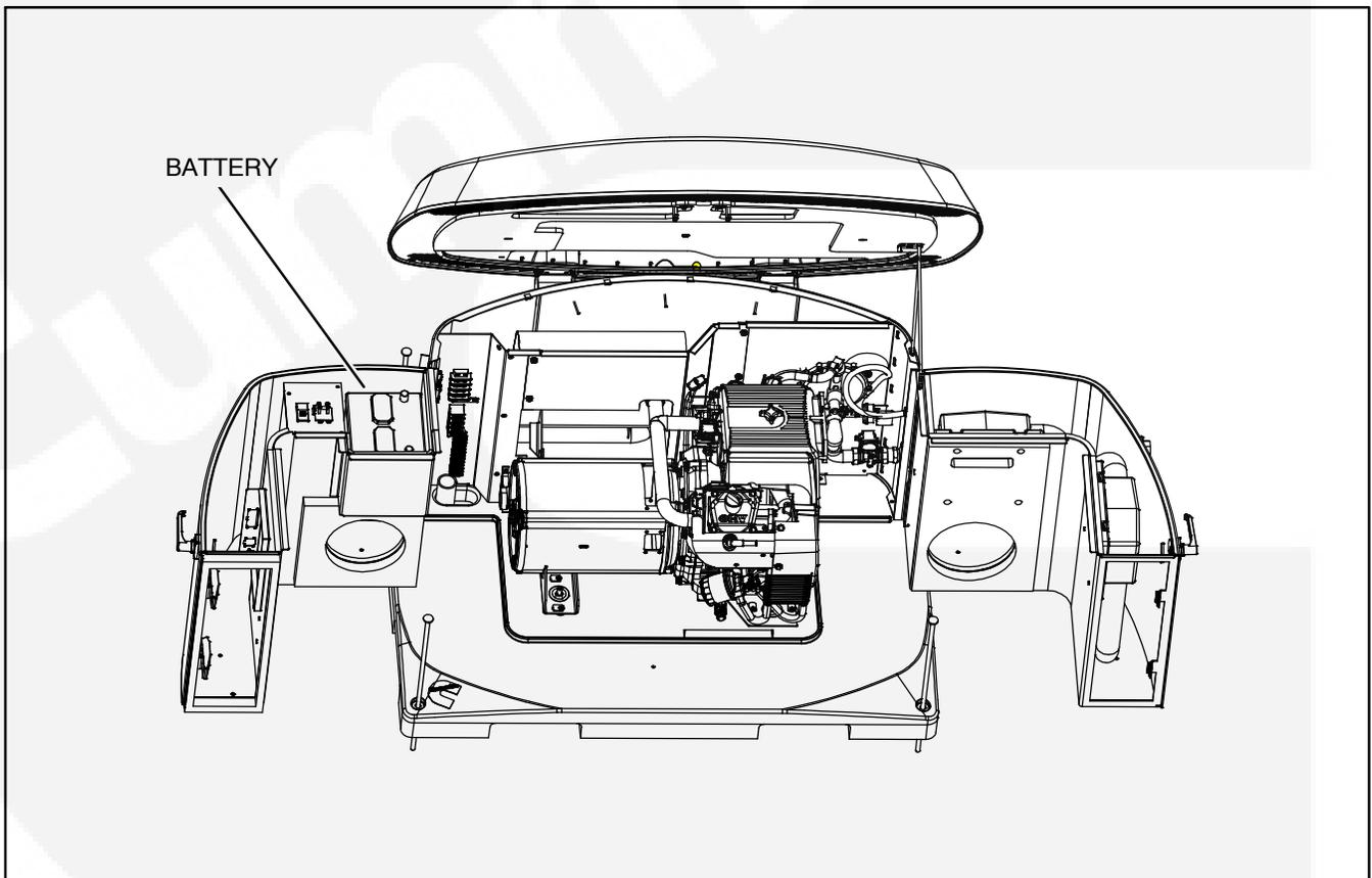
FIGURE 4-10. BATTERY INSTALLATION
