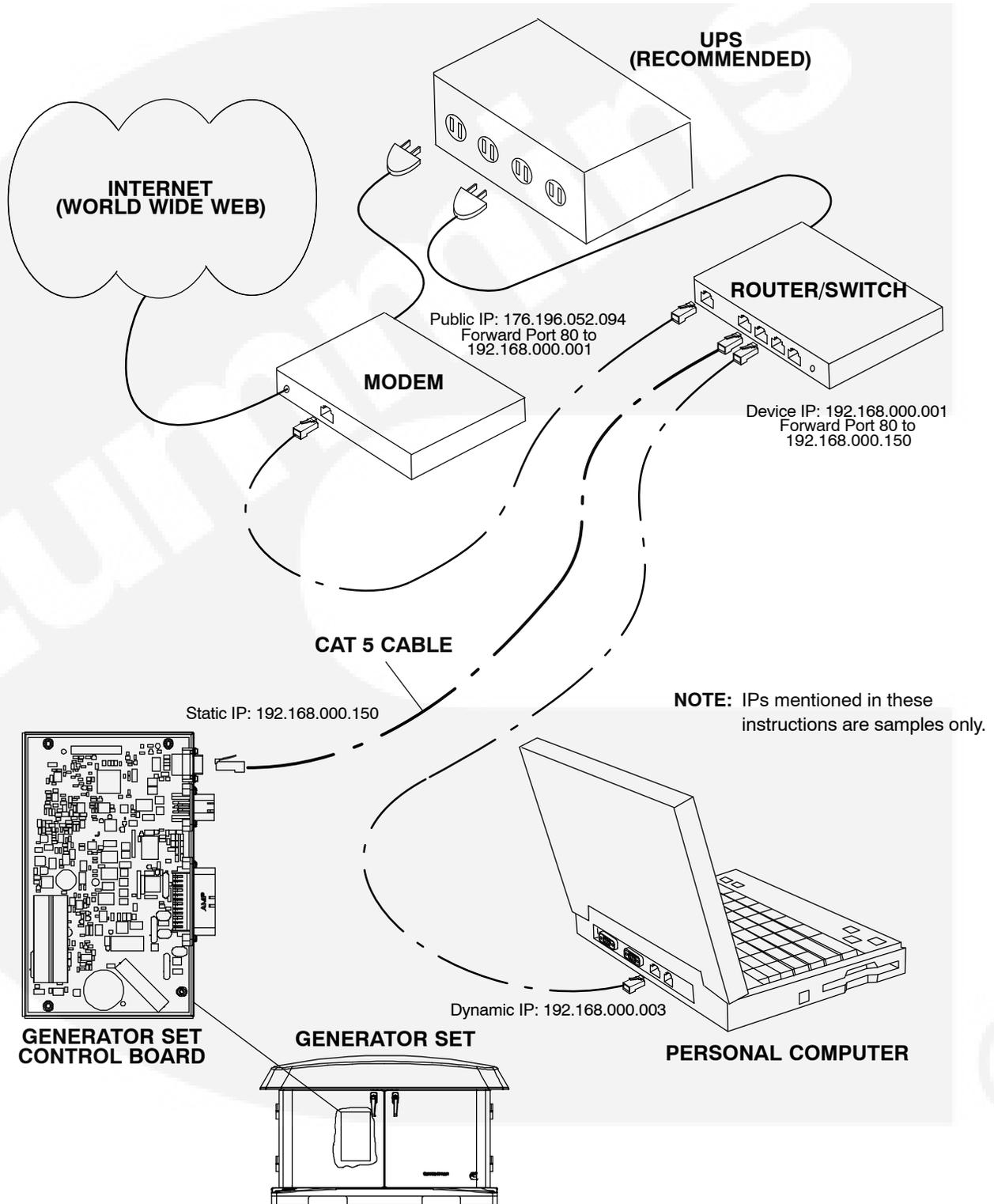
FIGURE C-1. NETWORK CONNECTIONS
