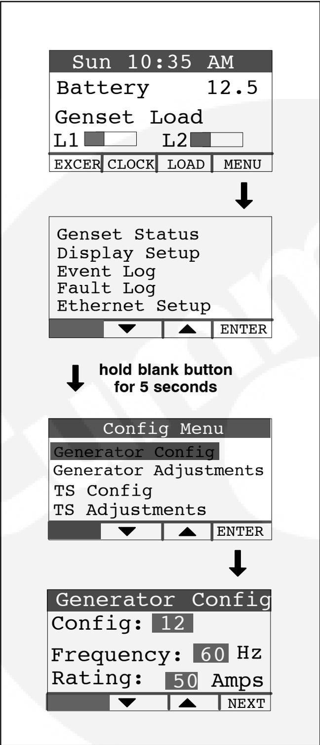
FIGURE 5-1. GENERATOR CONFIGURATION
