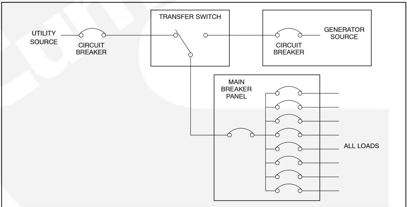
**FIGURE 4-6. FULL COVERAGE LOAD CONNECTIONS (TRANSFER SWITCH WITH CONTROLLER)**
