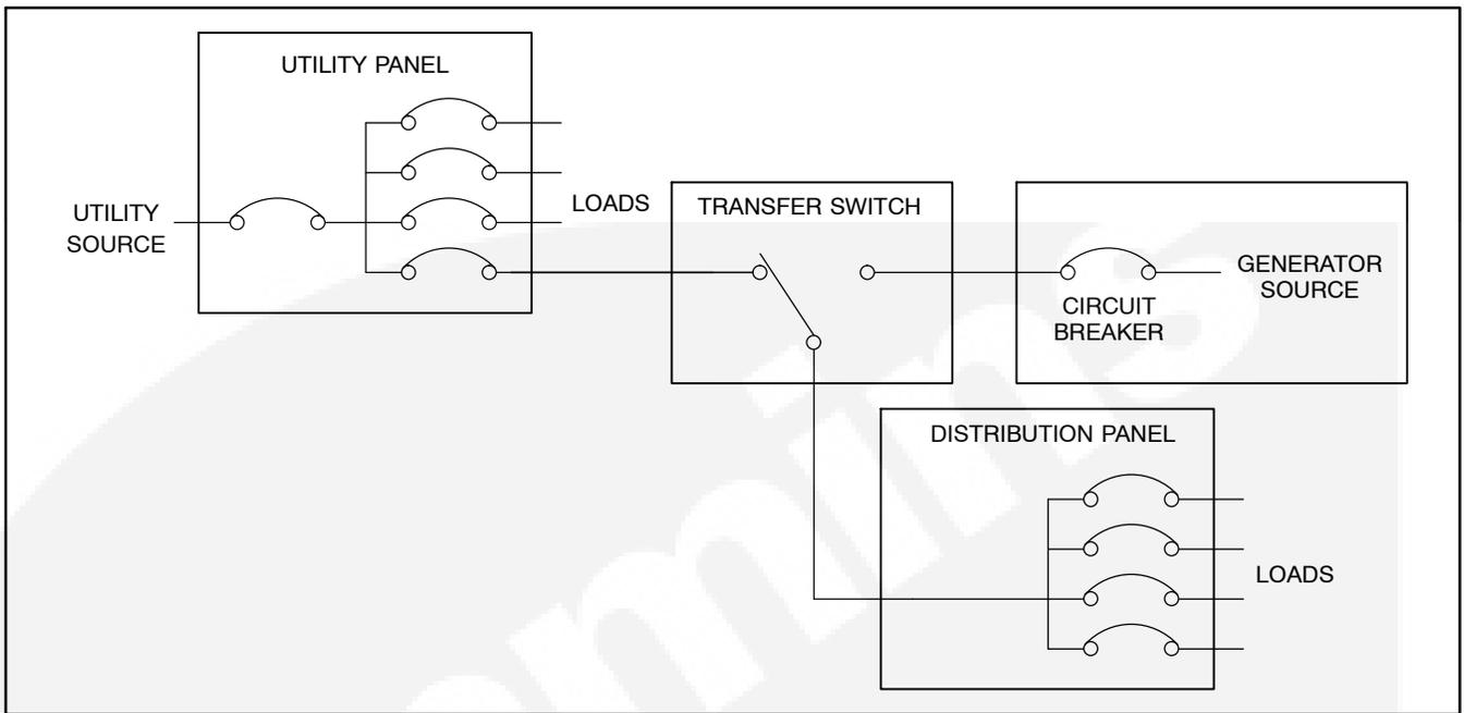
**FIGURE 4-5. PARTIAL COVERAGE LOAD CONNECTIONS (TRANSFER SWITCH WITH CONTROLLER)**
