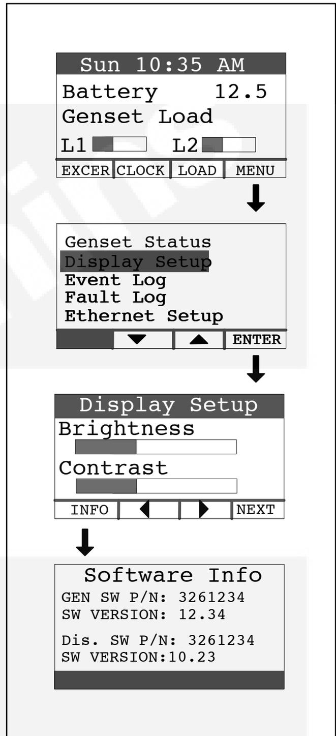
FIGURE A-9. DISPLAY SETUP AND SOFTWARE INFO SCREENS
