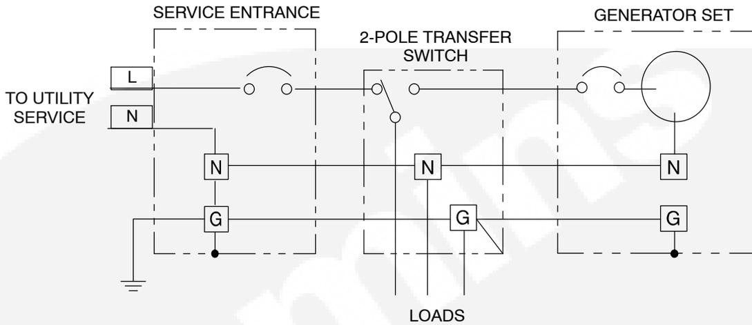
**GROUNDING WITH MODEL RSS 100-6868 AND RSS 200-6869 TRANSFER SWITCHES**
