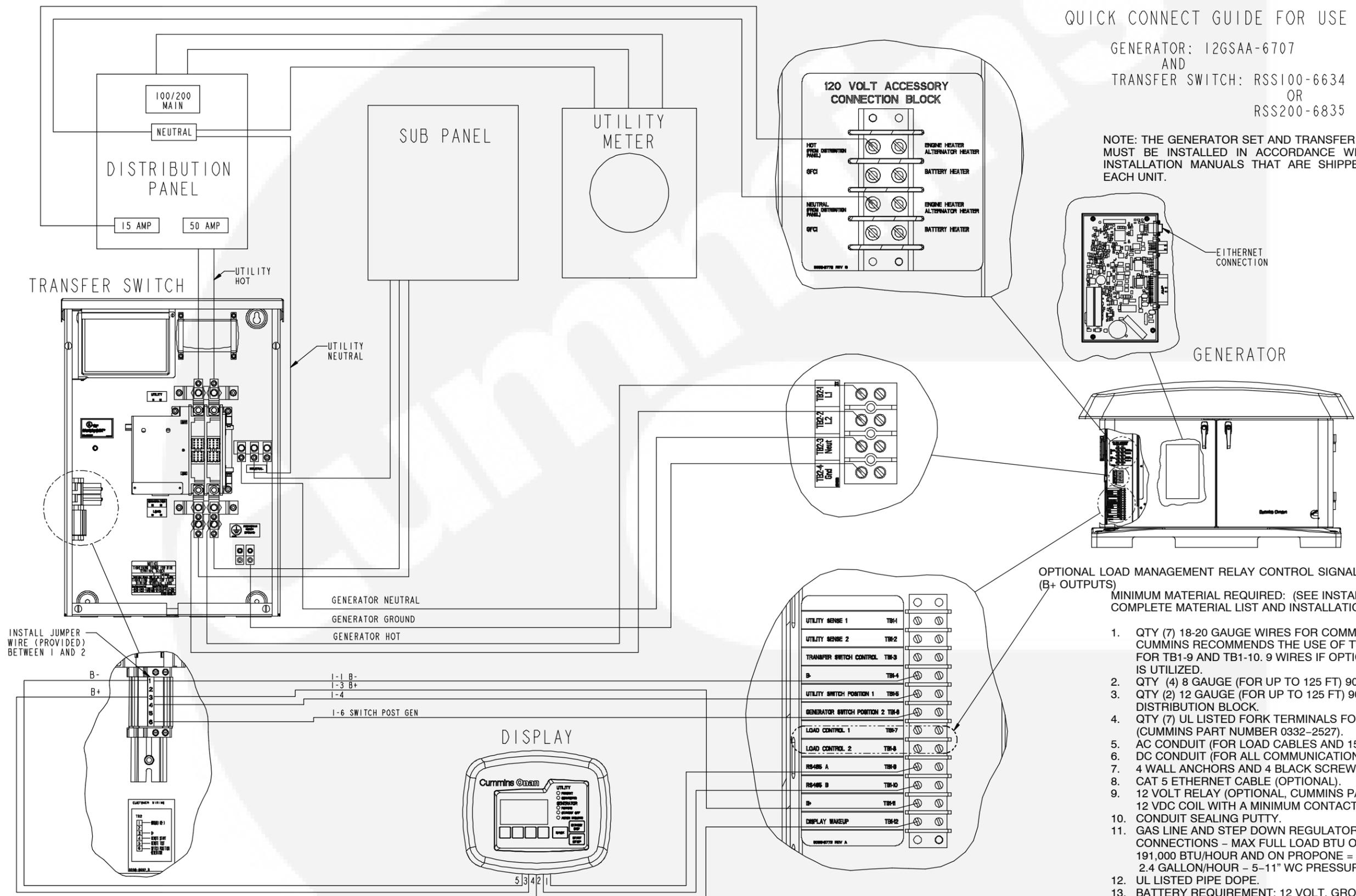
OPTIONAL LOAD MANAGEMENT RELAY CONTROL SIGNAL (B+ OUTPUTS)
