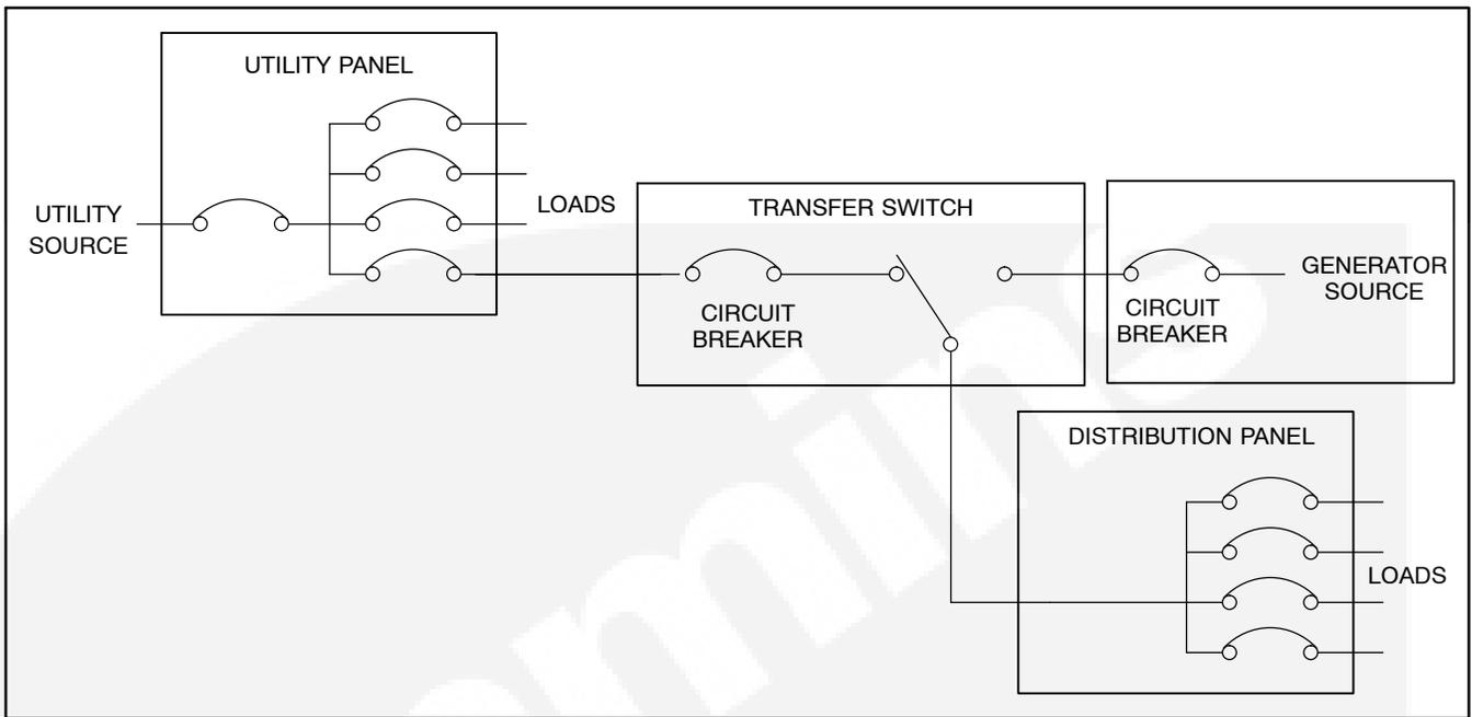
**FIGURE 4-3. PARTIAL COVERAGE LOAD CONNECTIONS (TRANSFER SWITCH WITHOUT CONTROLLER)**
