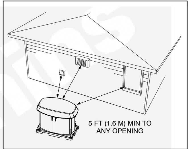
FIGURE 2-2. GENERATOR SET CLEARANCES
