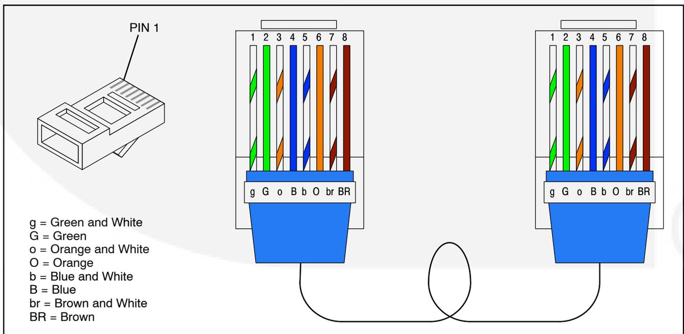
FIGURE 4-9. ETHERNET RJ-45 CONNECTOR WIRING
