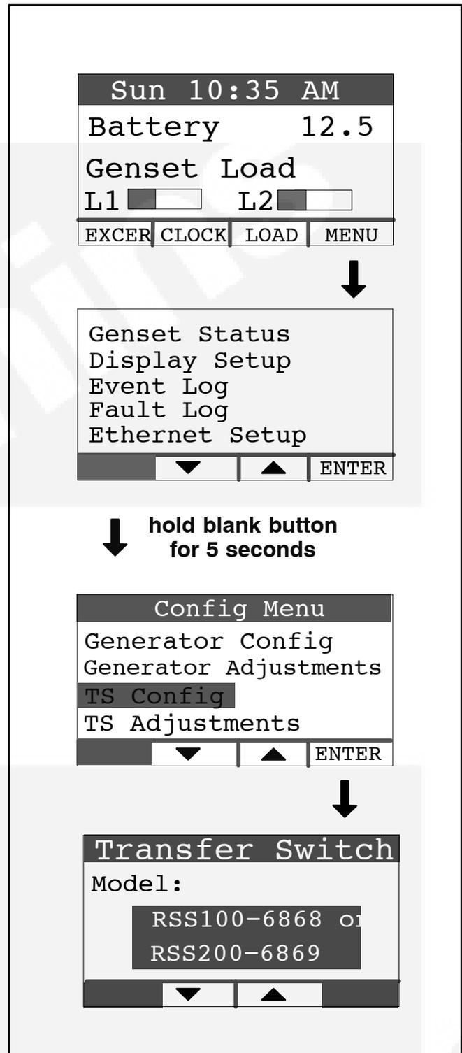
FIGURE 5-4. TRANSFER SWITCH CONFIGURATION
