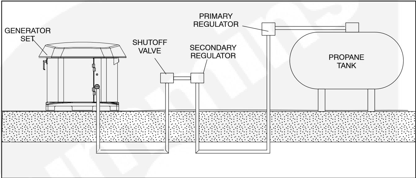
FIGURE 3-4. TYPICAL PROPANE VAPOR WITHDRAWAL INSTALLATION
