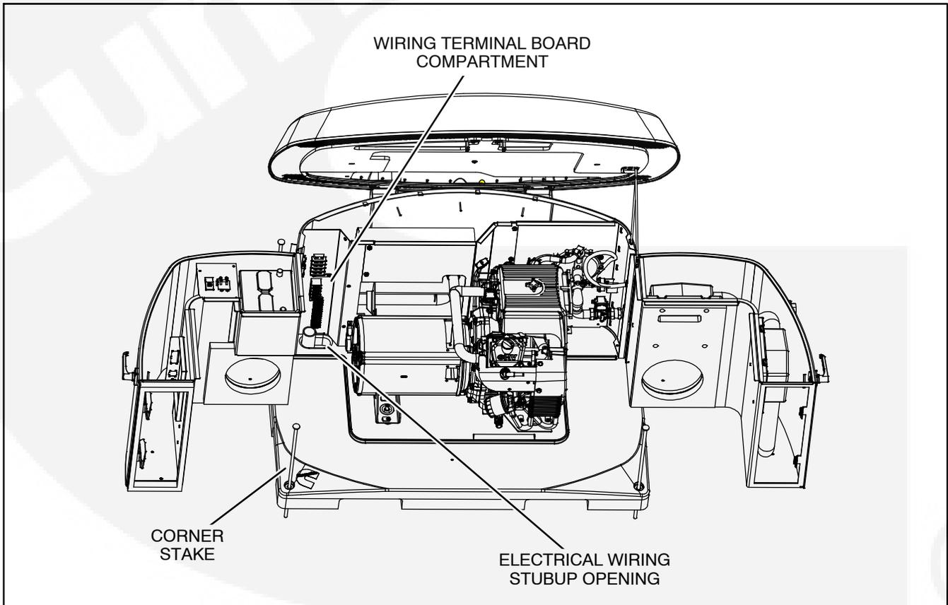
FIGURE 2-3. ELECTRICAL WIRING TERMINAL BOARDS AND STUBUP OPENING
