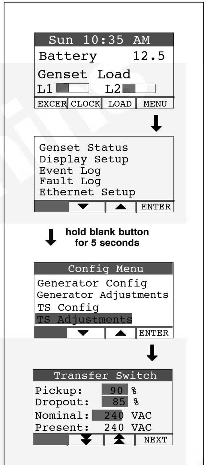
FIGURE 5-5. TRANSFER SWITCH ADJUSTMENTS
