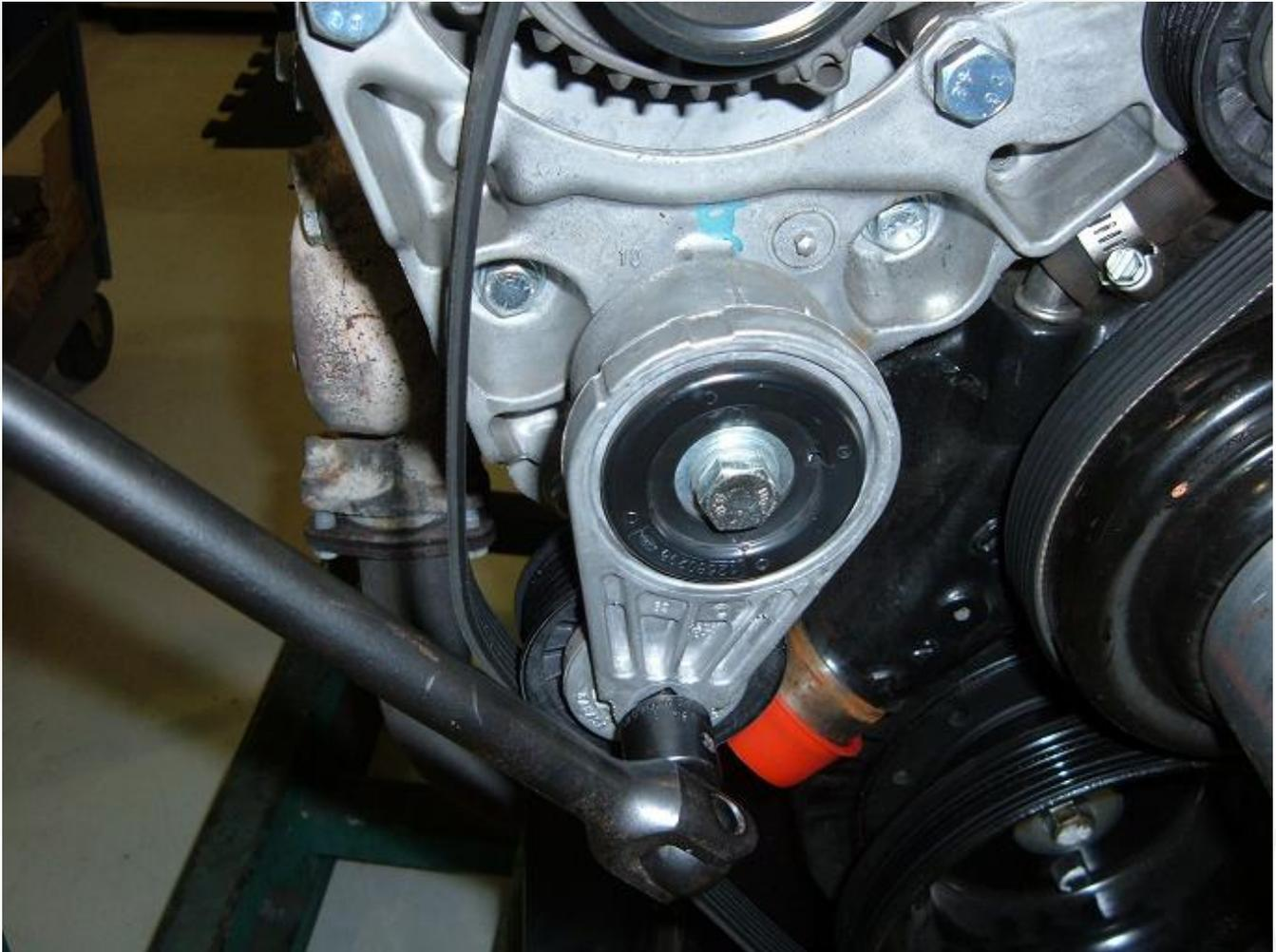
**FIGURE 25. BELT REPLACEMENT WITH RATCHET INSERTED IN TENSIONER**
